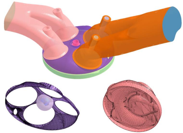
Figure 1. Model 3D mesh. The ball around the spark plug location identifies the refined meshing zone.
