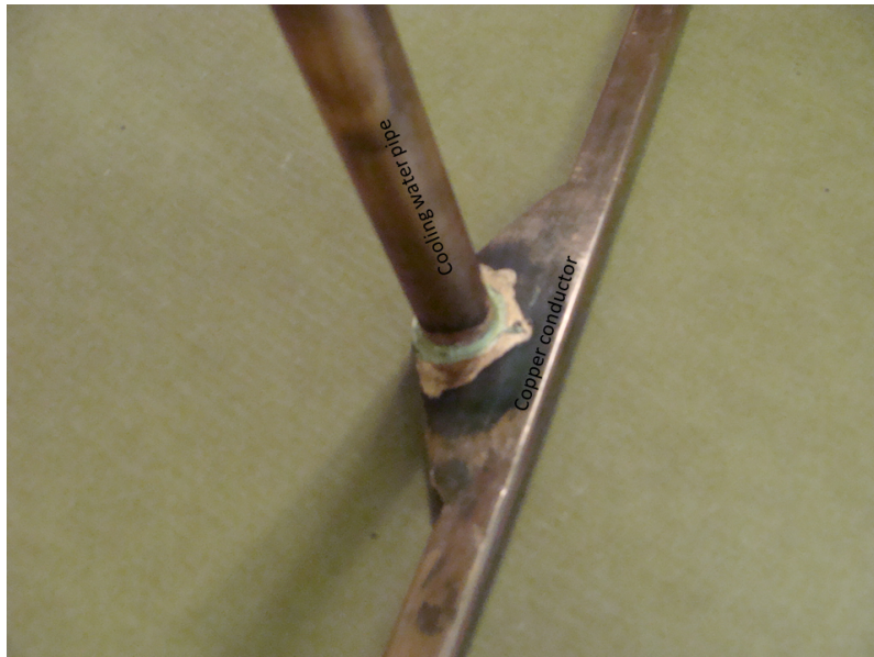
Figure 22: A picture of the brazing connection of one of the cooling pipes with one of the four conductors of the coil.
