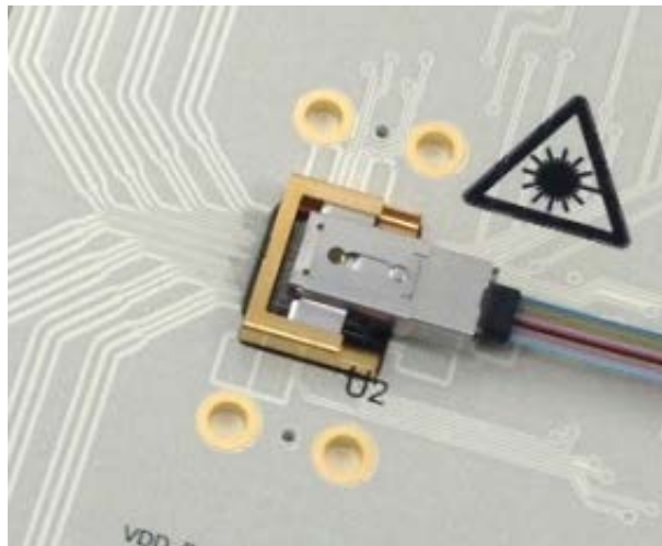
Figure 20: CSP transceiver mounted to test board.
