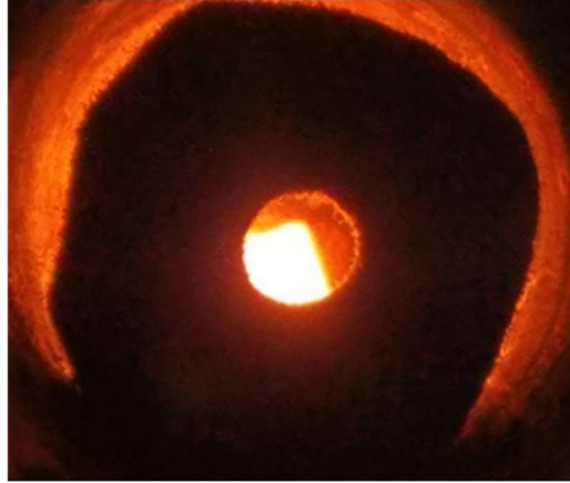
Figure 3.39: View from pyrometer port of the U_3Si_2 tile for calibration testing
