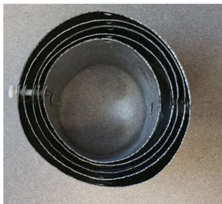
Figure 3.24: Heat shield top view. The sample is contained in the middle
