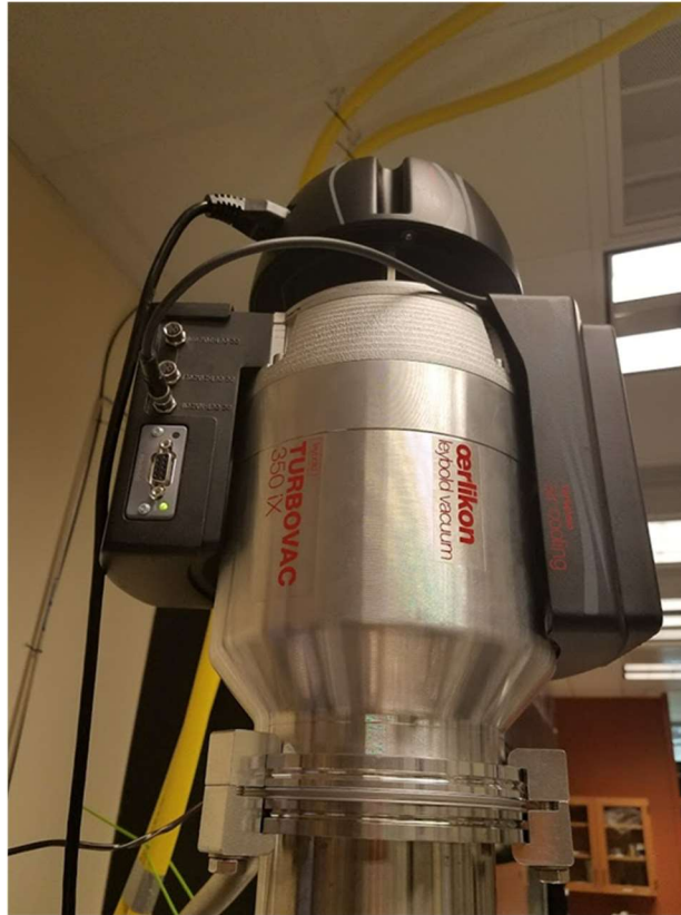
Figure 3.33: Turbomolecular pump to bring system to high vacuum
