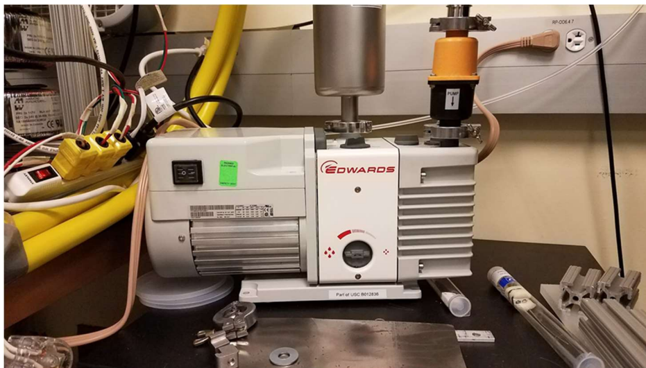
Figure 3.32: Roughing vane pump for low vacuum
