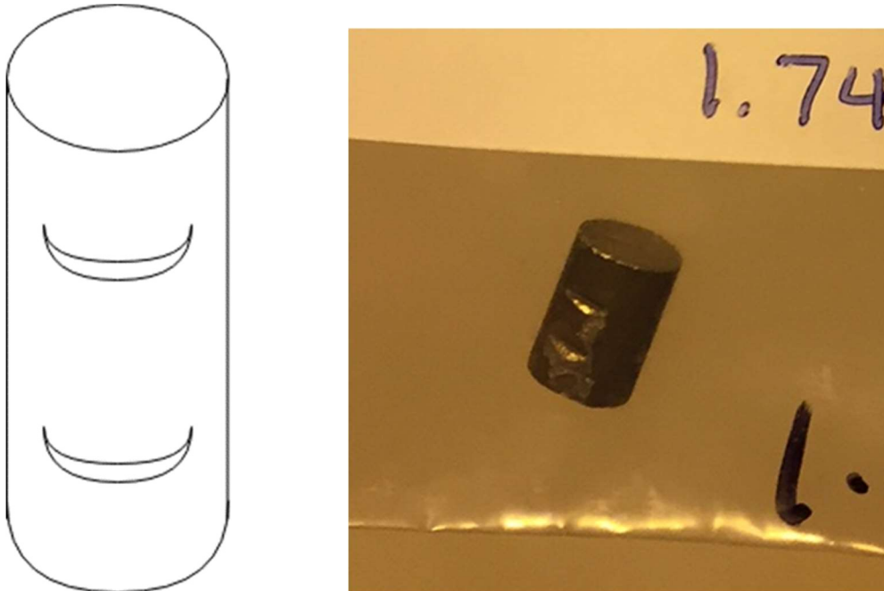
Figure 3.3: Sketch of a notched sample (left) with a typical creep sample (150813a) on the right
