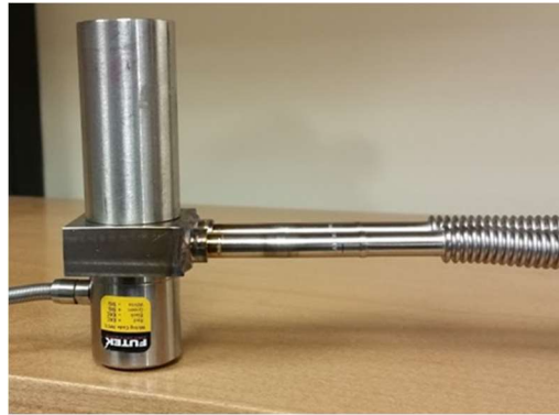
Figure 3.15: Load cell assembly with water pass through
