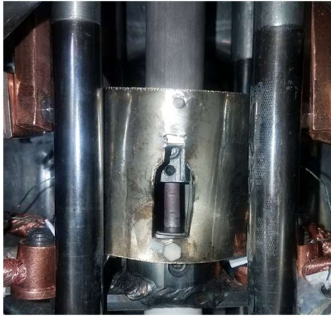
Figure 3.25: Radiation shield as installed in testing chamber
