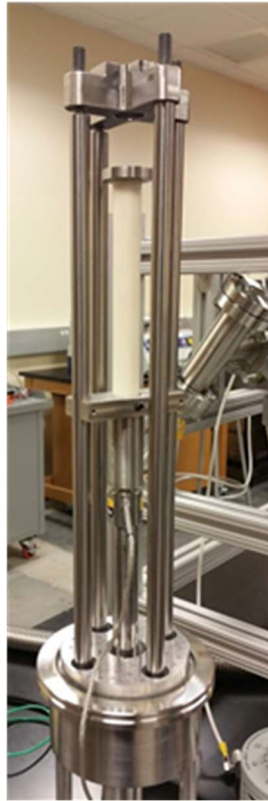
Figure 3.13: As constructed internal loading frame
