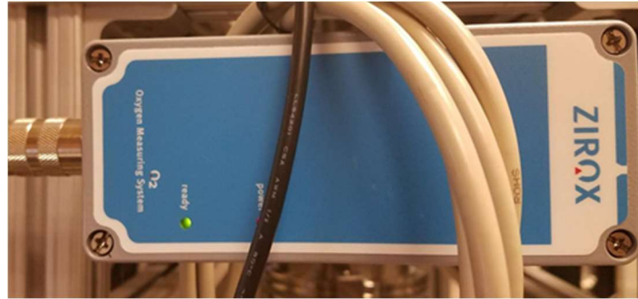
Figure 3.34: Zirox oxygen partial pressure probe
