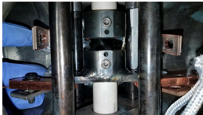
Figure 3.21: Inconel platens as installed in testing chamber
