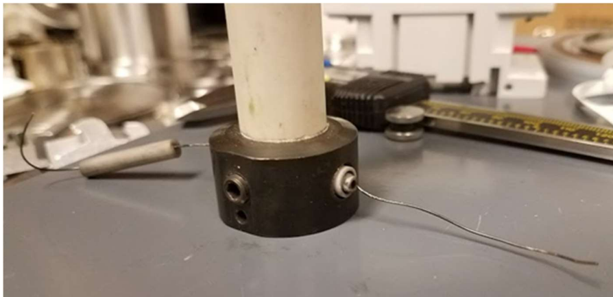
Figure 3.30: Cartridge heaters inserted into top platen
