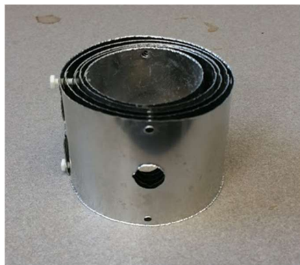
Figure 3.23: Stainless steel heat shield with viewing holes
