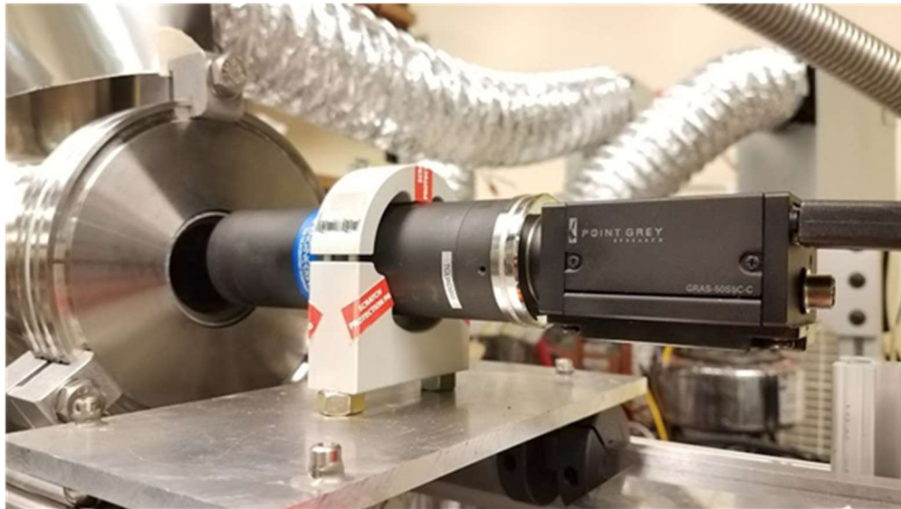
Figure 3.41: Camera as focused on the sample outside of the test rig
