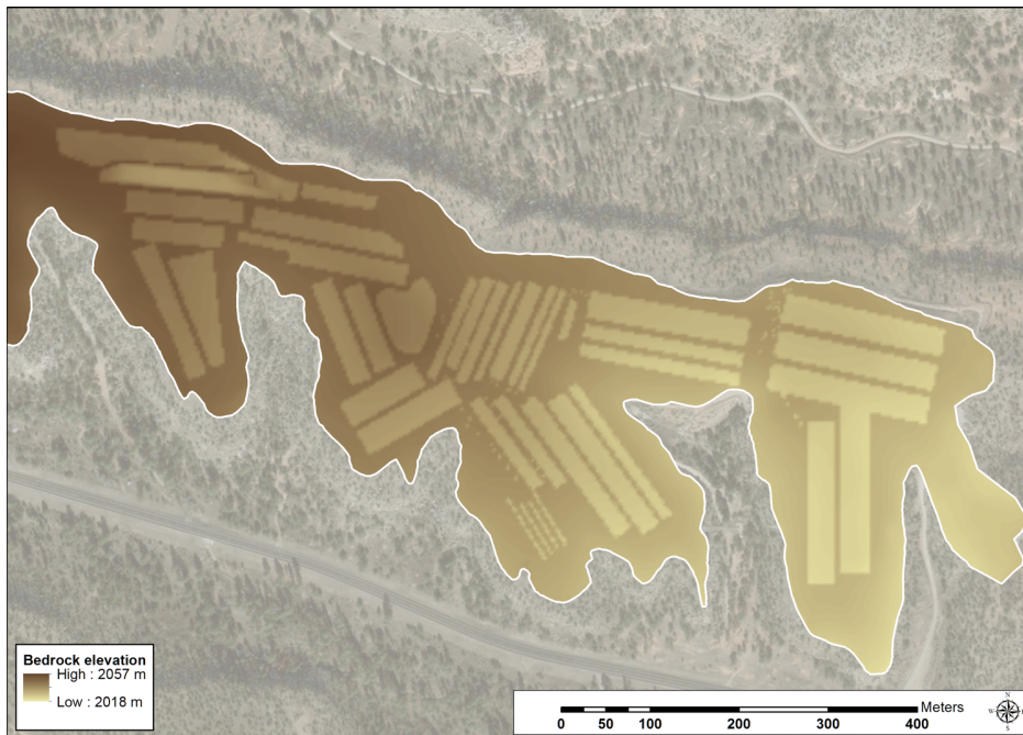
Figure 2-9. Bedrock elevation with waste pits etched in, used for SIBERIA calculations.
