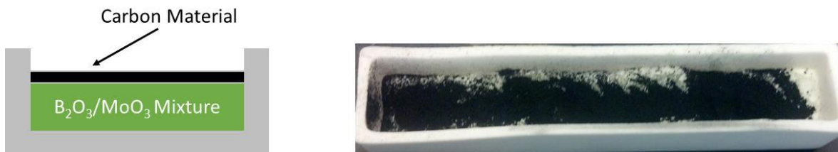
Figure 4: Diagram and picture of the crucible with the reactants inside.
