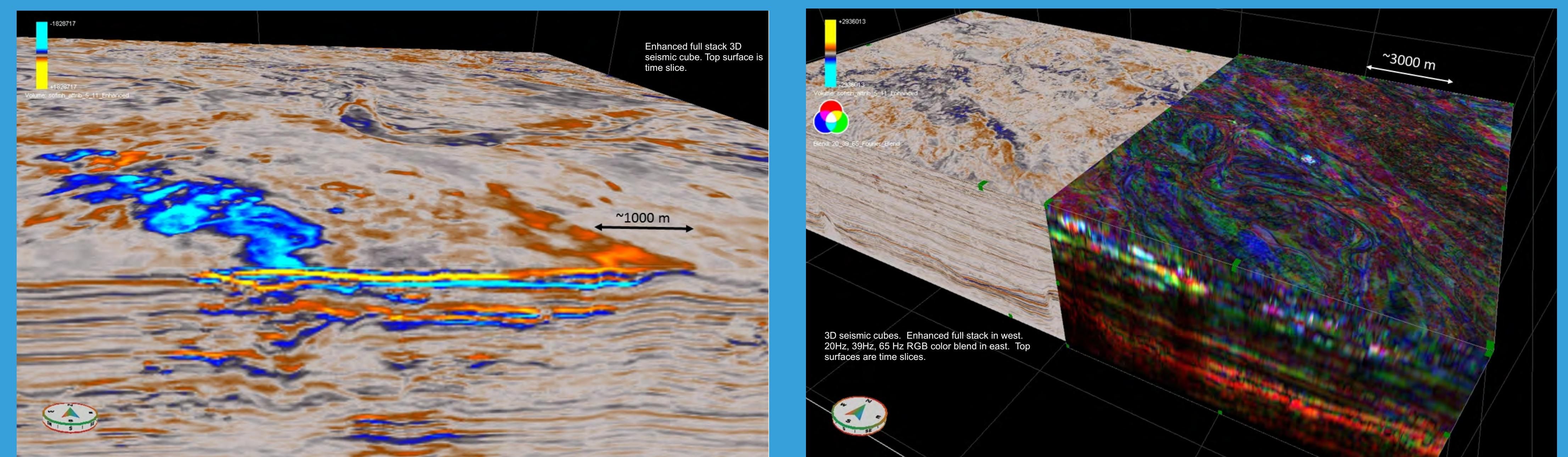
RGB blend of 20 Hz, 39 Hz, and 65 Hz narrow band frequencies from Fourier transform shows high frequency dominance in the interpreted gas hydrate deposit and low frequency dominance in the gas leg.
