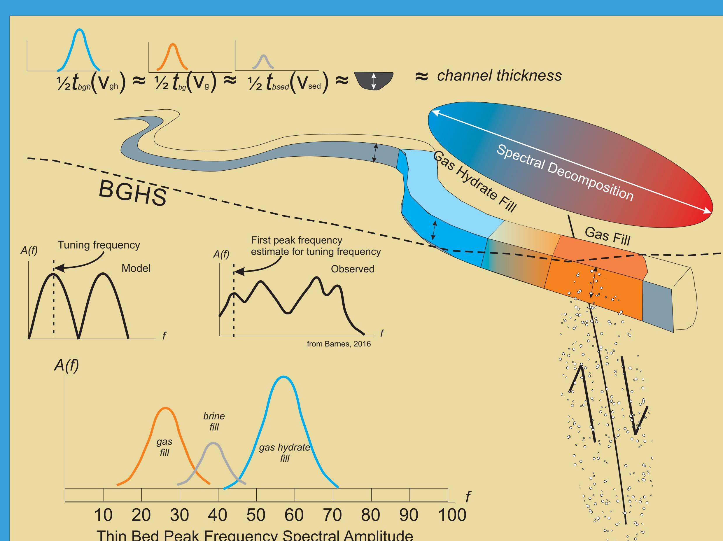
Spectral decomposition is primarily a tool to determine thin bed thickness. Using it in that strict way, the channel with gas hydrate is thinner in time than the channel with no hydrocarbon charge and the channel is thickest in time where it is gas filled.
