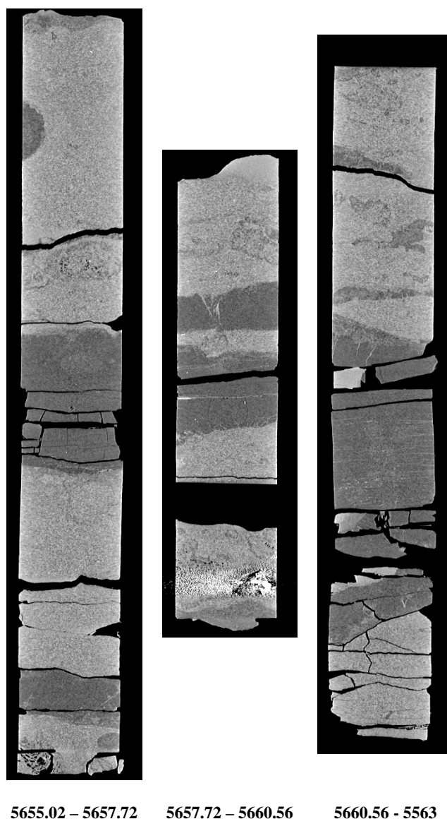
Figure 19: Tippens 6HS, medical CT scans from 5655.02 to 5563 ft.
