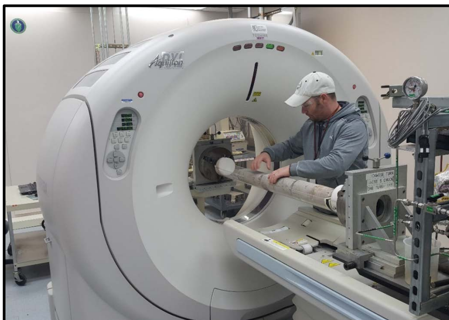
Figure 11: Toshiba® Aquilion™ Multislice Helical Computed Tomography Scanner at the NETL used for core analysis.
