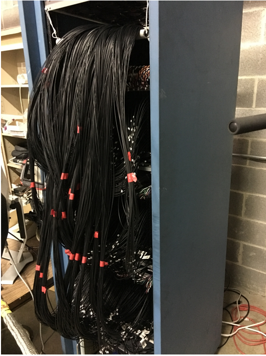
(a) Camera1 1024 fiber connections to electronics boards.
