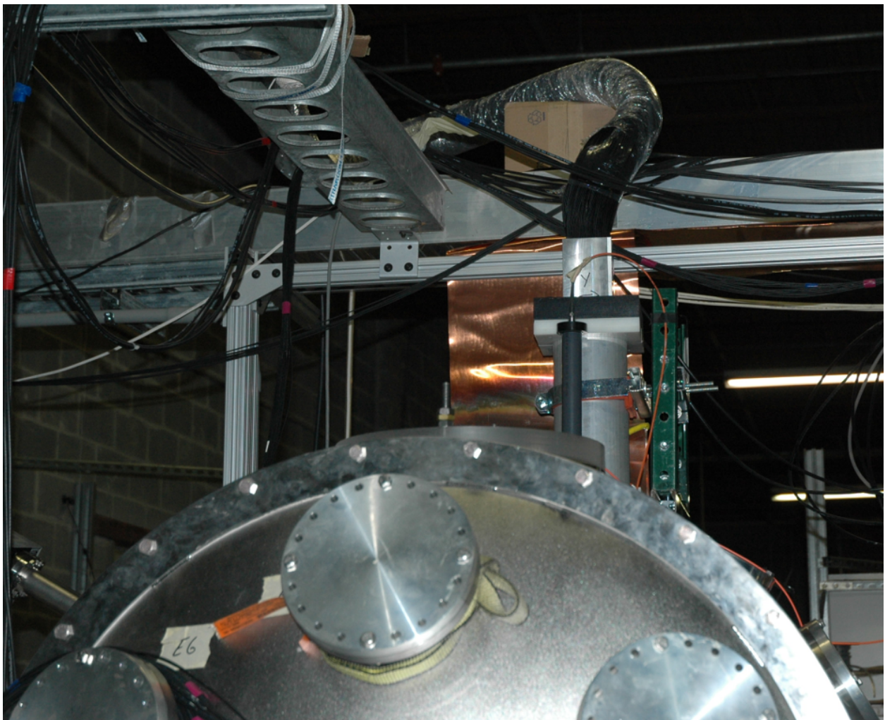
Figure 20 A set of collection optics was used to image visible plasma emission on to the 32 x 32 fiber imaging grid. These collection optics were mounted on the first window looking down into the chamber about 35 cm from the nose of the plasma accelerator.
