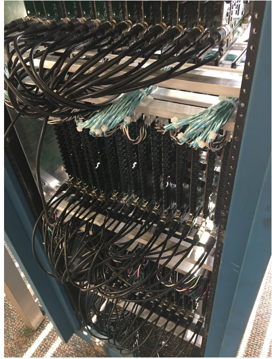
(b) Camera2 circuit boards prior to fiber connections.
