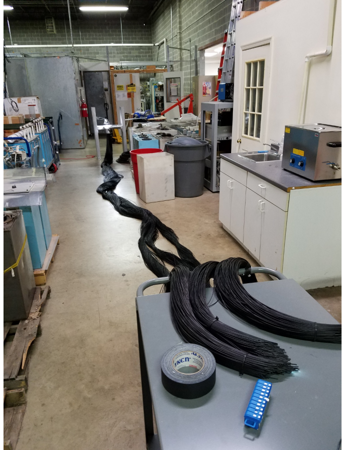
Figure 15 We constructed a mask that would leave one column or row exposed to illumination (Left). We then mounted the fiber grid under a bright lamp so that the mask could be scooted across the grid face in the x and y directions. We then set out the fiber bundles to be sorted (Right). A row was illuminated and the 32 fibers lit the brightest were bundled together and marked as that row number. All 32 rows were sorted and labeled this way. Then the mask was turned 90 degrees and a column was illuminated. The brightest fiber in each bundle was then labeled as that column number. Thus in 64 moves of the mask, the course x and y location of each fiber was determined.
