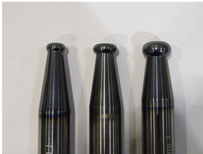
Figure 3.6 Flat-tip forming tools. Tip sizes are 12 mm by 6 mm, 15 mm by 6 mm, and 18 mm by 10 mm, respectively
