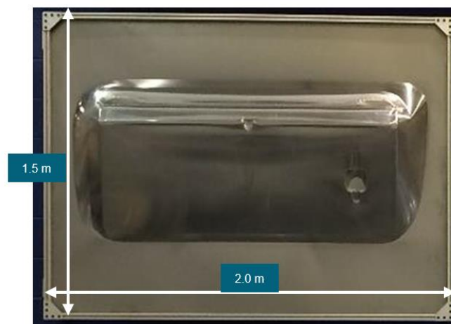
Figure 1.2 RAFFT formed panel
