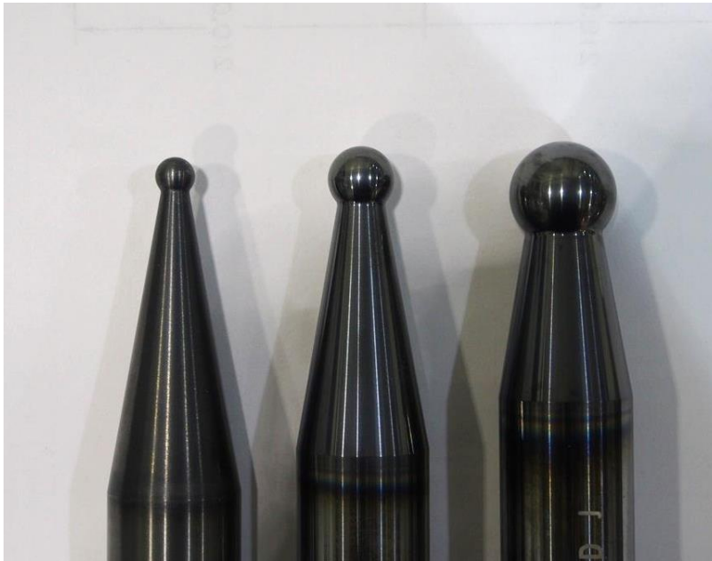
Figure 3.5 Ball-tip forming tools. Tip diameters are 6 mm, 10 mm, and 16 mm
