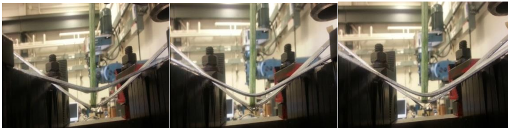
Figure 3.44 Effect of pulse duration on part springback under v-bend testing conditions (left to right: 2, 3, and 4 second pulse durations at 40A/mm 2 )
