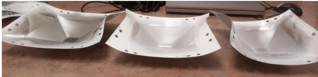
Figure 3.42 Effect of step down size on final part geometry (from left to right - 0.85mm, 0.55mm, 0.25mm step down sizes)
