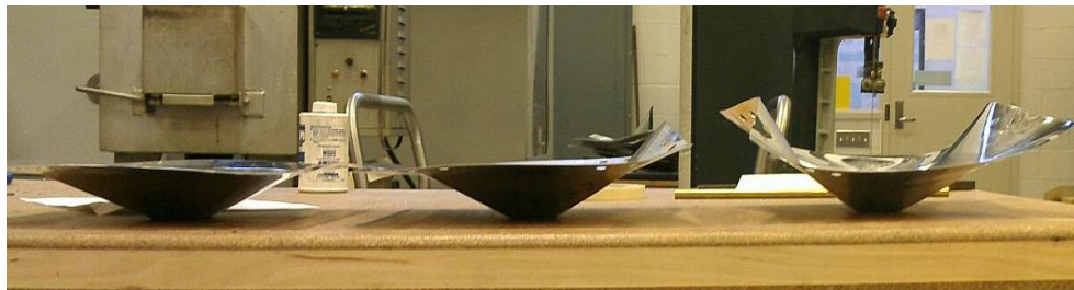
Figure 3.43 Examples of varying part distortion due solely to Clamping Configuration
