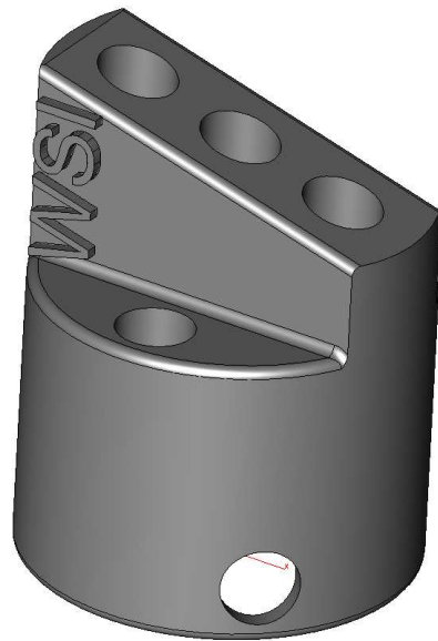
Alumina Langmuir probe head with cooling channels and WSI logo - less expensive than without!
