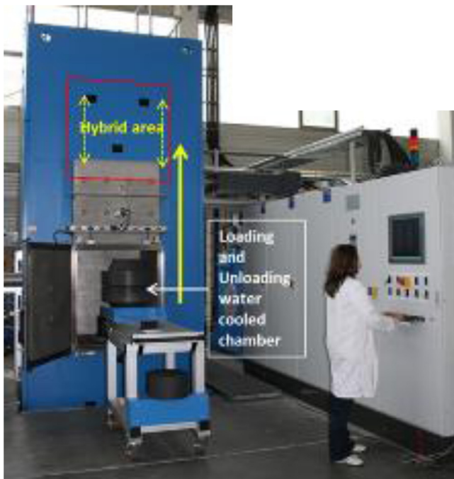
Fig. 5. Industrial scale hot press used for Field Assisted Sintering at the Applied Research Lab at Penn State University.
