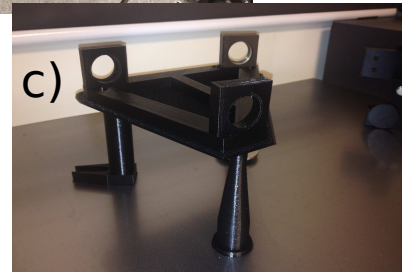
a) original interferometer components; b) pre-aligned monolithic mirror mounts; c) printed monolithic assy
