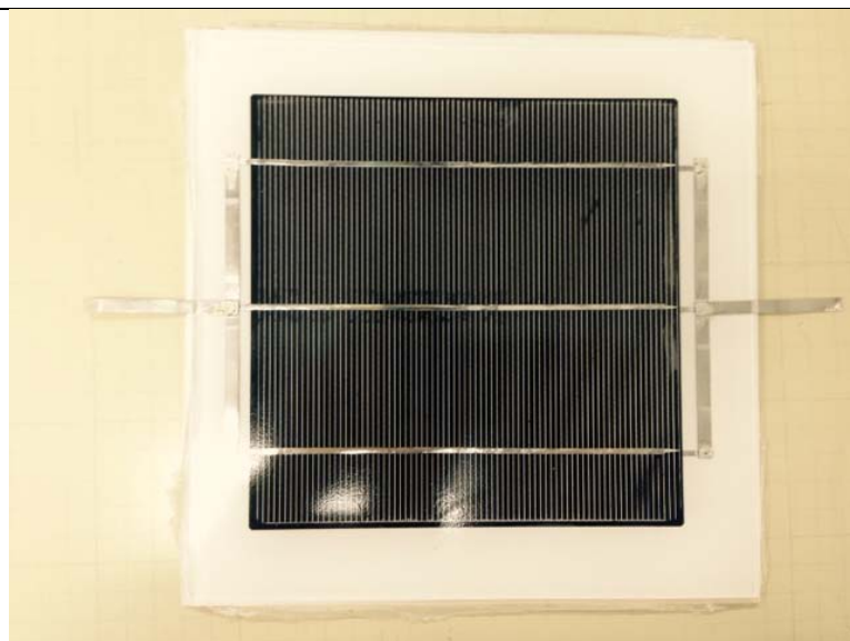
Figure 3: Picture of encapsulated solar cell with plated nickel, copper, and tin front grid metallization.
