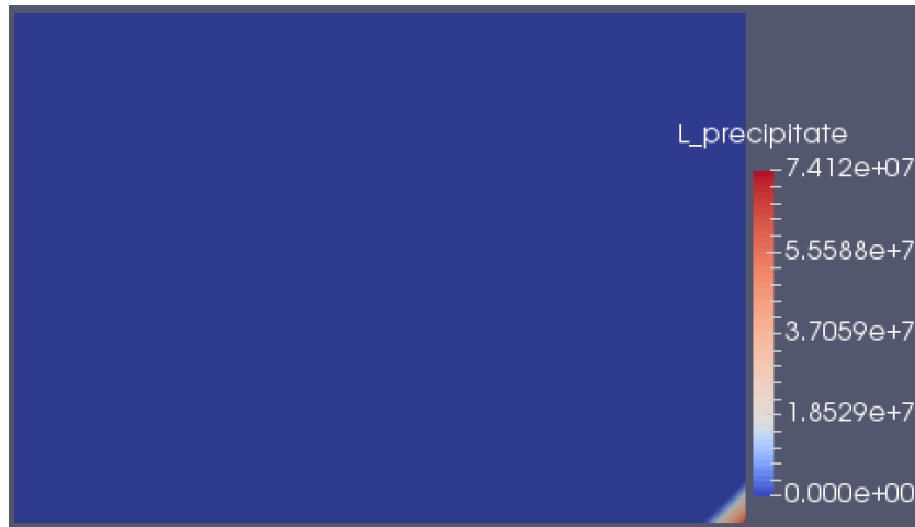
Figure 73 Distribution of Ce precipitates concentration in liquid metal solution with a 2-D temperature profile as indicated in Figure 72. The Ce generation rate is set to 7.9399 \text{ atoms}/\mu\text{m}^3/\text{s} in the fuel blocks.
