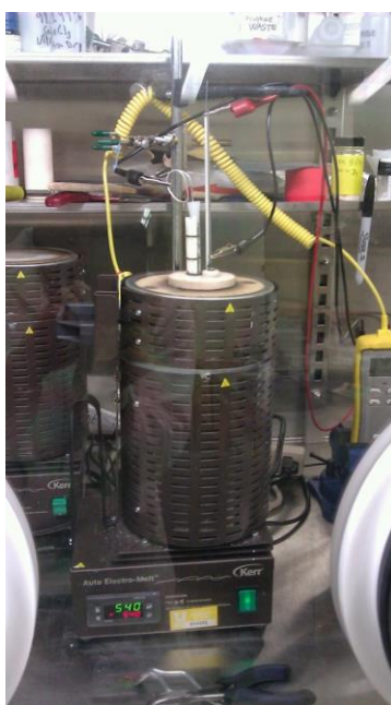
Figure 3-3: Kerr electromelt furnace used for melting salts in the NPML gloveboxes.
