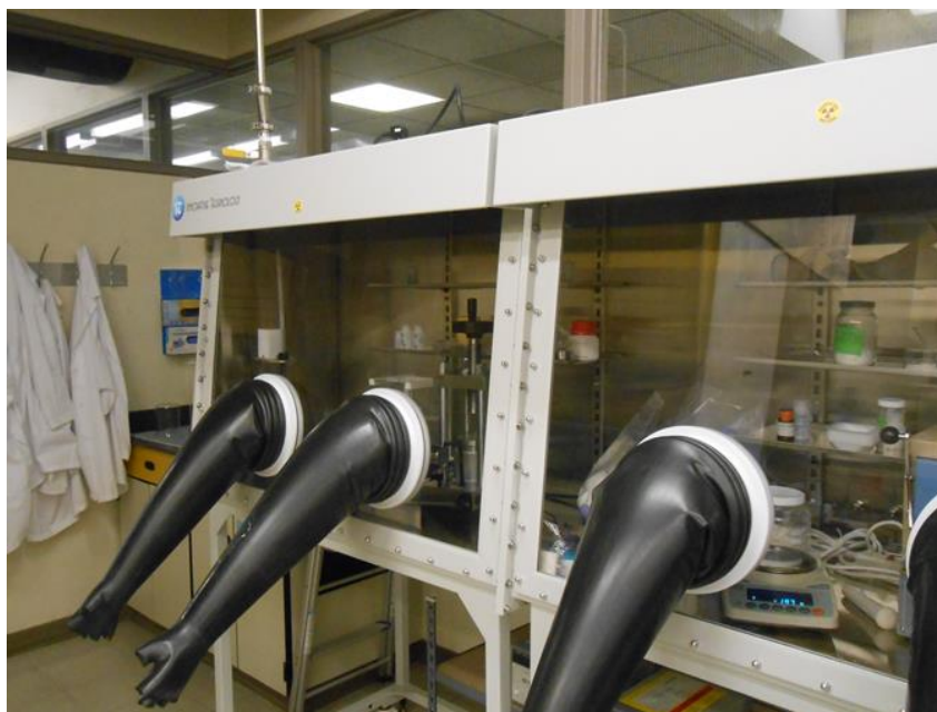
Figure 3-1: Argon atmosphere glove box and high temperature electrochemistry furnace.
