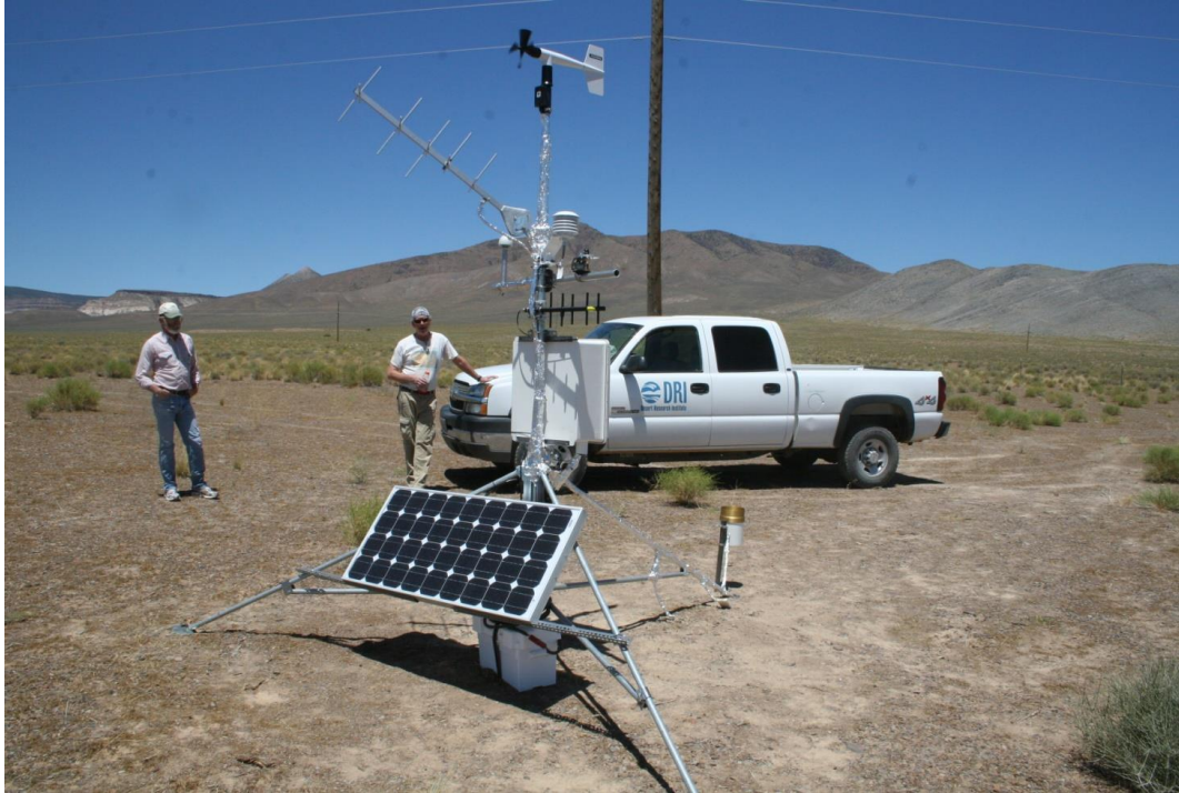
Figure 3. The Smoky Site CA meteorological station was installed to measure precipitation, wind, and other climate parameters.
