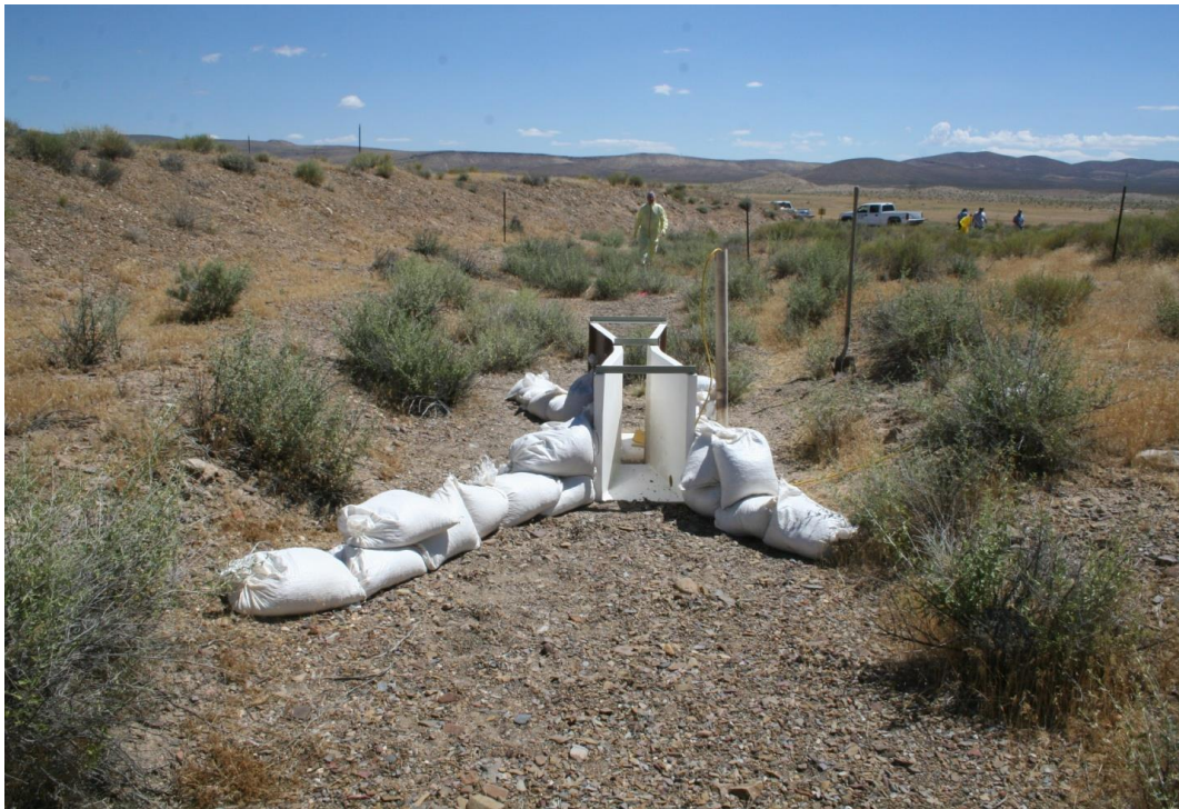
Figure 4. View looking downstream through the Parshall flume installed to measure runoff from the Smoky Site CA (prior to washout in July 2013).
