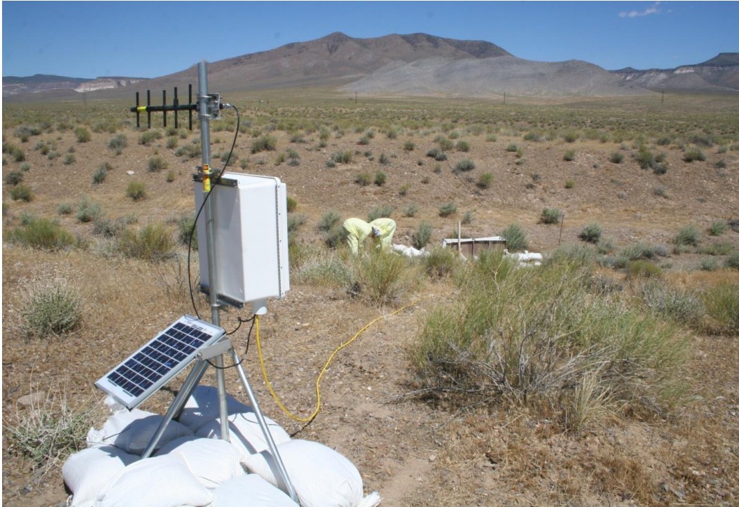
Figure 5. Runoff conditions in the flume are detected by the pressure transducer (yellow cable), recorded in the datalogger (white box), and relayed by radio (black antenna) to the meteorological station for transmission to the WRCC via the GOES.
