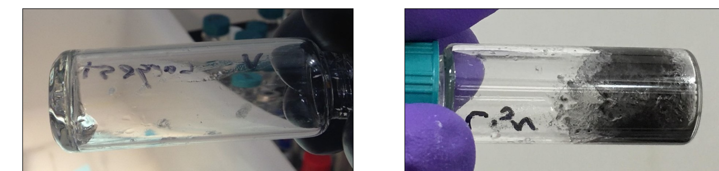
Figure 3. Reaction of (left) \text{VX} + \text{LiAlH}_4 and (right) \text{HD} + \text{Li}_3\text{N} + \text{H}_2\text{O}
