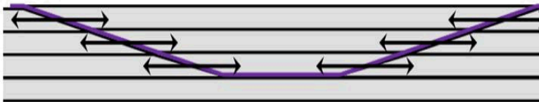
Scarfed Blade Repair Process
