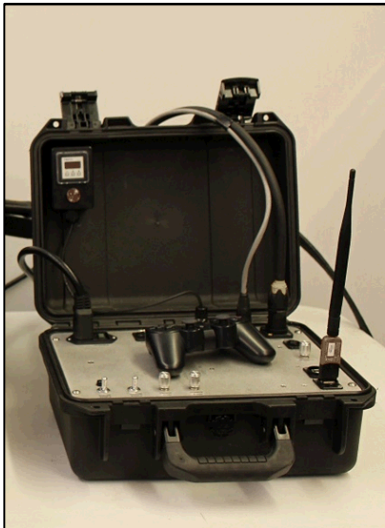
Ground Workstation – Data Acquisition & Analysis Plus Control of Robot
