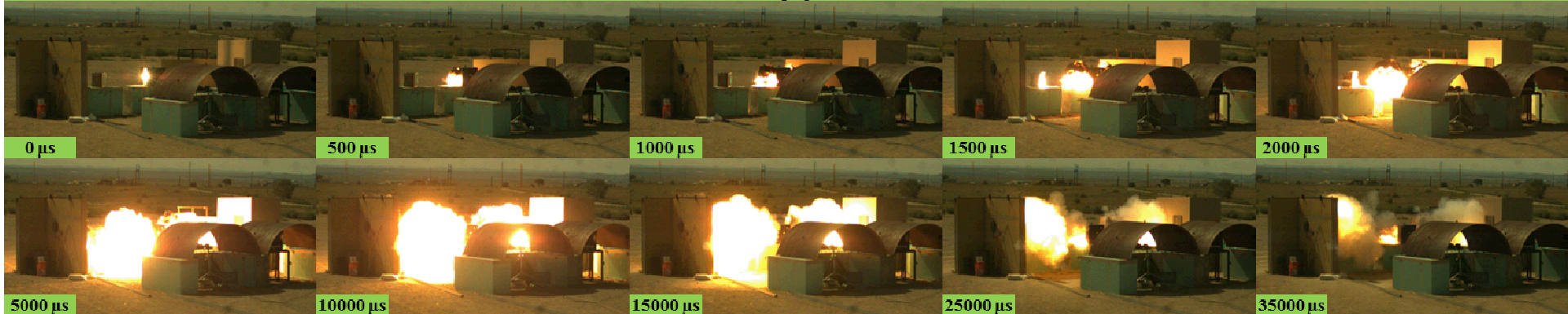
Test 11: 0.3" wall, high-pressure, embrittled aluminum
