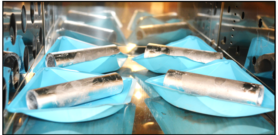
Al cylinders in oven with Ga application
