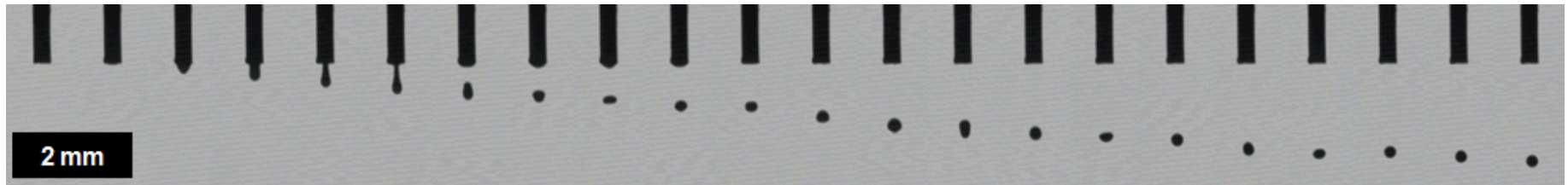
Strobe-illuminated photographs of Al/Bi 2 O 3 ink droplet formation. 100 μs between images.
