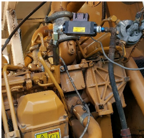
Figure 2: Return line KRAL flowmeter installed during rig move.
