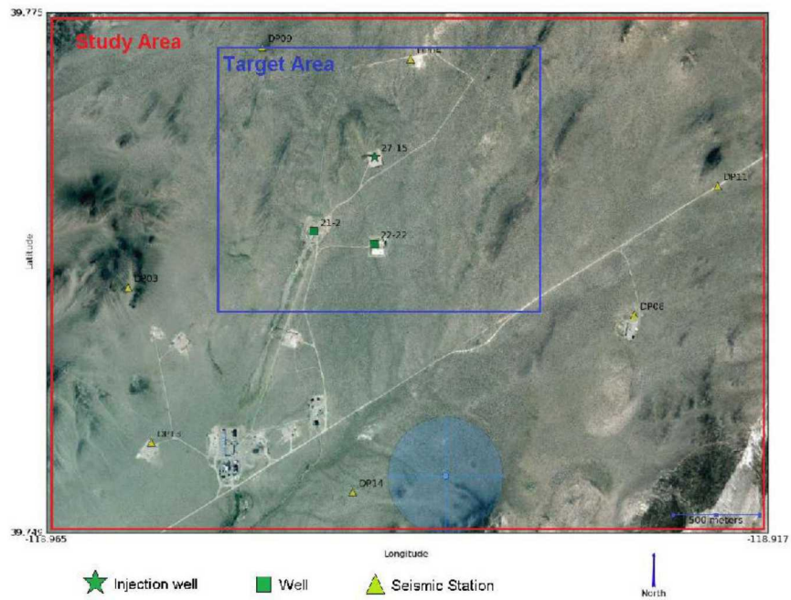
Figure 13. The surface outline of the 12 km 3 Desert Peak EGS target area, which is centered on the target well (27-15).
