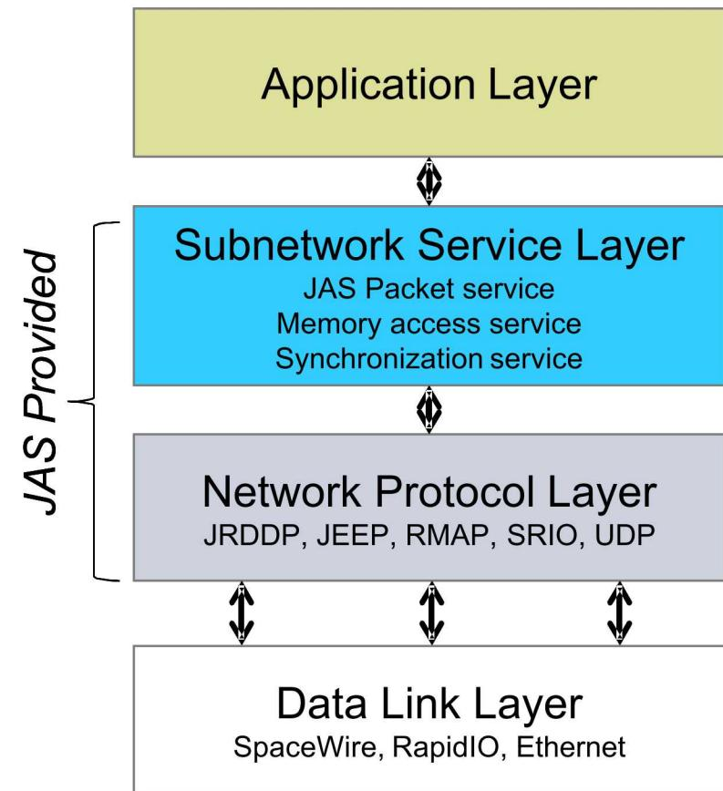
*JAS supports a layered architecture that facilitates application reuse*
