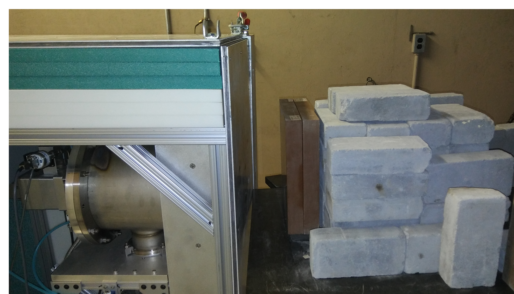
Fig 3: DD110M neutron generator (Adelphi Technology, Inc.) uses a DD reaction moderated by aluminum and shielded with borated polypropylene to irradiate air sampler filters for activation analysis.
