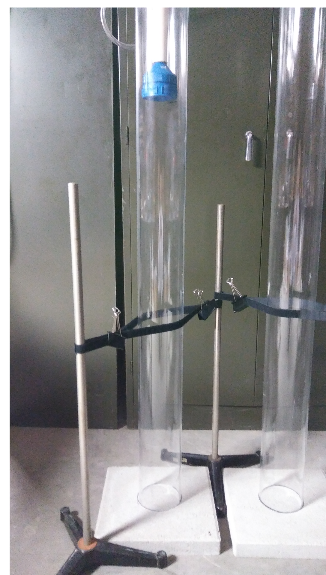
Fig 2: In-house resuspension chamber used to experimentally probe resuspended concentrations of powder atop concrete within an acrylic tube.
