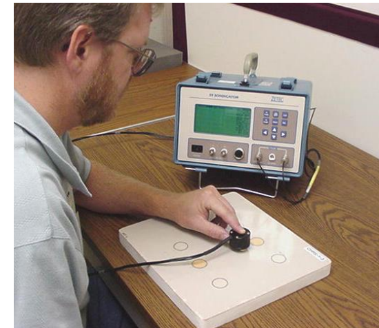
Corrosion Detection with Dual Frequency Eddy Current
