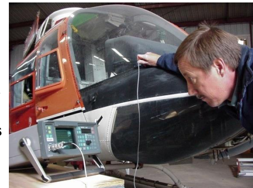
Corrosion Detection with Dual Frequency Eddy Current
