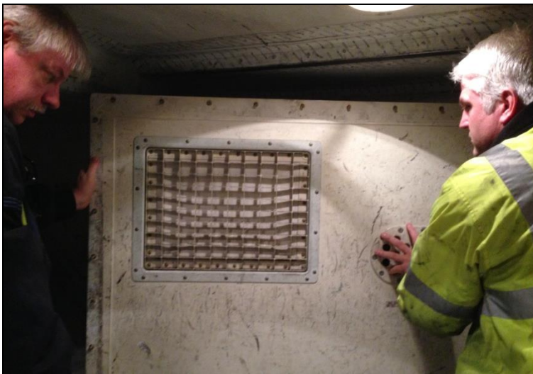
Removal of Baggage Liner to Access 4 SLS Connectors Mounted to Bulkhead
