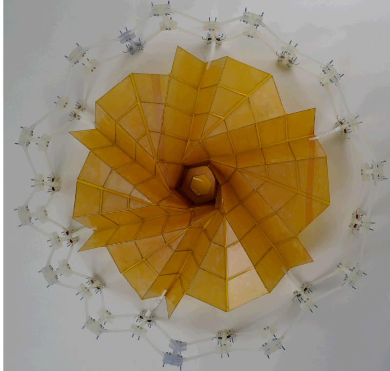
Partially opened model of the HanaFlex array and truss. Zirbel et al 2015
