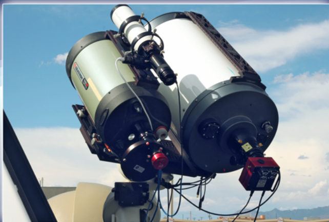
Fig. 3 Photograph of the variety of hardware Sohbrit can use including telescopes, robotic filter wheel, cameras, and focuser
