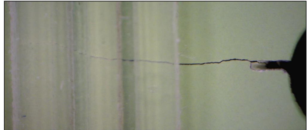
Cracks viewed under load to track growth and show engagement with CVM galleries
