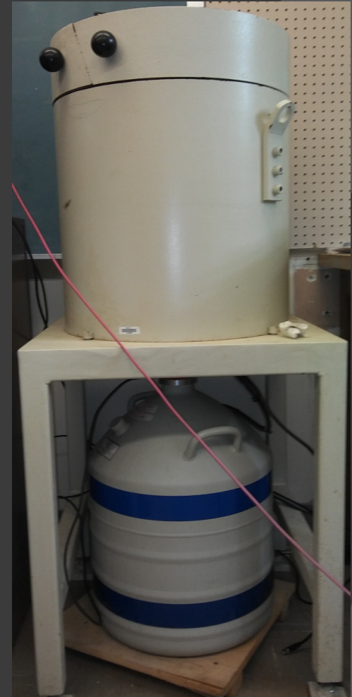
Figure 7: Broad energy Li-drifted Ge detector system with Cd shielding at WPI.
