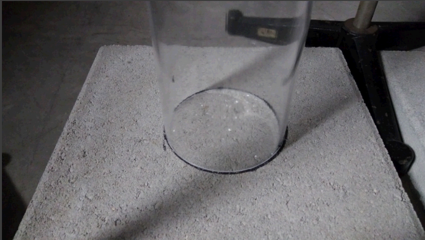
Figure 4: Close-up of particulate deposits on concrete surface following air release.
