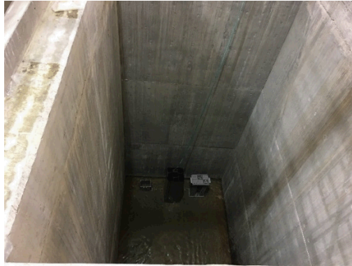
Figure 4: Floor vault as it is filled with water. Left object is facility equipment, center is the BWR storage rack with a mockup BWR assembly, right is facility equipment with two metal plates containing engraved characters on its top. Camera view is from opposite side of pool from targets.
