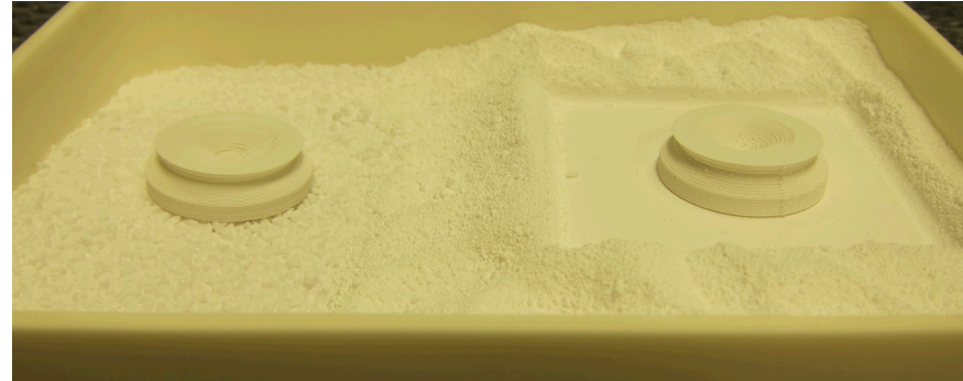
Parts in a crucible for de-binding and sintering
