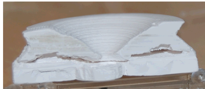
Cross-section of fractured ceramic sample
