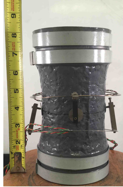
(a) Generalized schematic of the testing apparatus (not to scale). (b) Deformation gauges on deformed sample.
