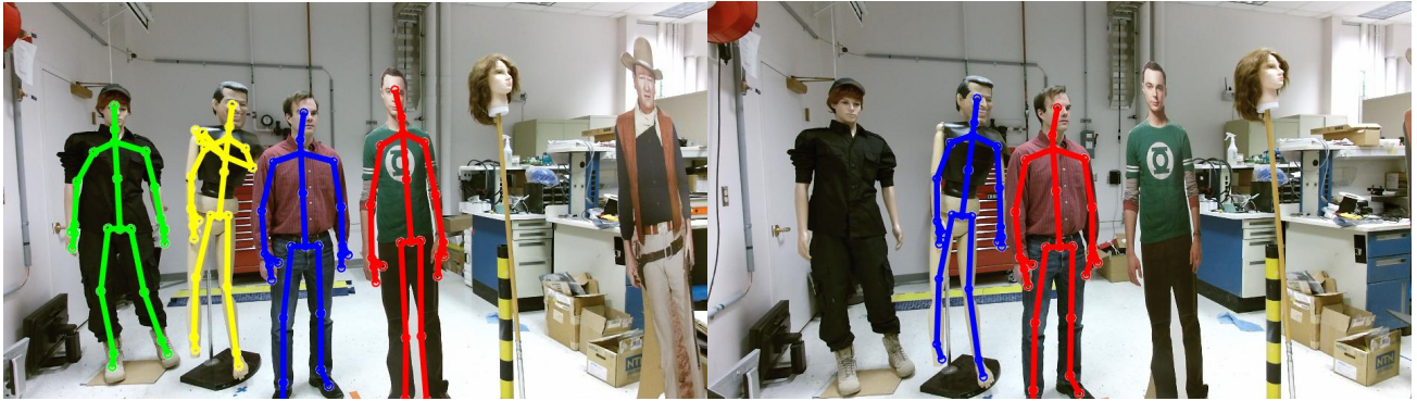
Figure 10. Skeleton tracking for the cardboard cutouts (e.g., Cooper) degrades as they are viewed from the side.
