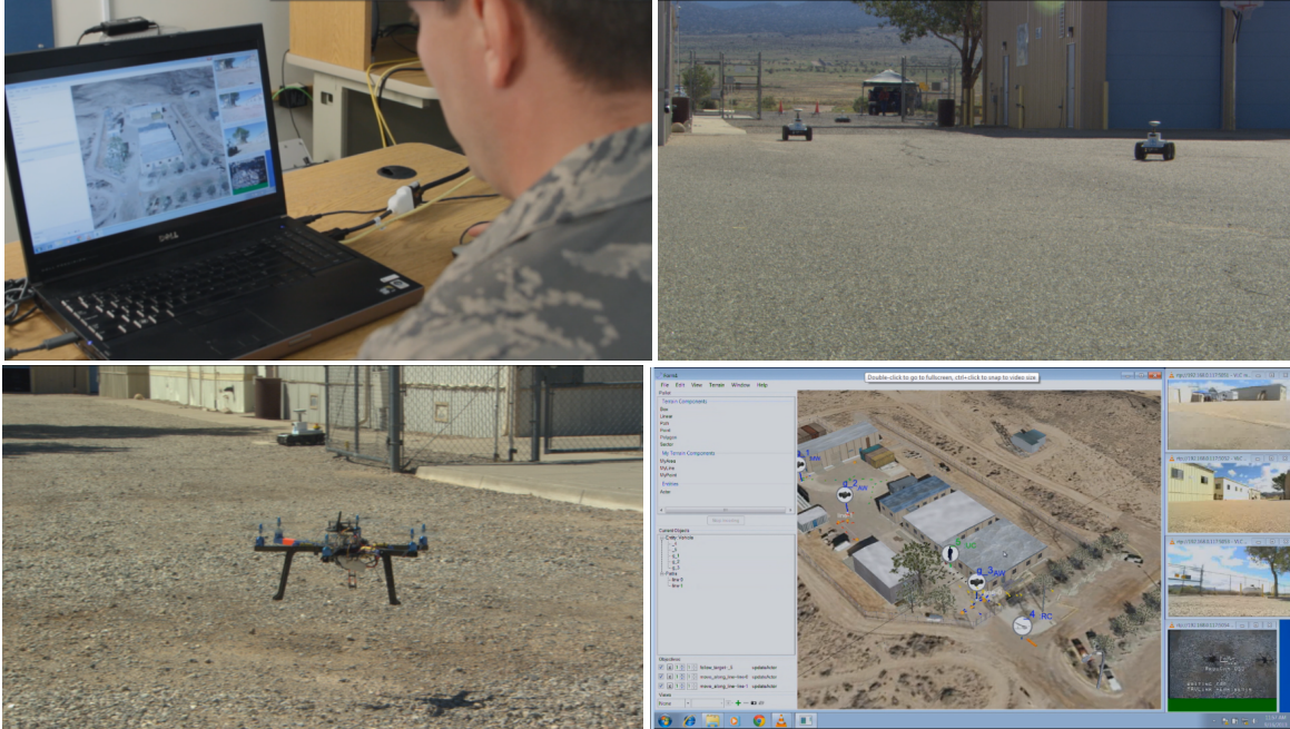
Figure 3. Screenshots from a demonstration of a single operator (top left) directing a heterogeneous team of four unmanned ground (top right) and air (bottom left) vehicles in a dynamic, tactical operation. The user interface (bottom right) includes live sensor feeds (right panels) a 3D common operating picture (middle), and a series of graphical tools that enable the operator to build missions in real-time in response to unpredictable observations and adversary behavior.
