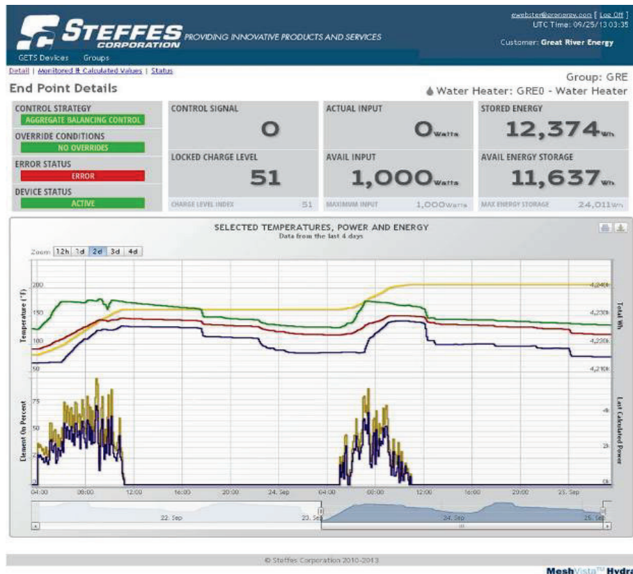
Figure 72. Steffes Data on Temperature, Power, and Energy for an Individual Water Heater
