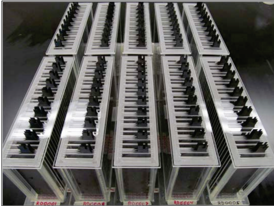
Figure 39. 1-kW Zinc-air Prototype (Photo courtesy of EOS Energy Storage)
