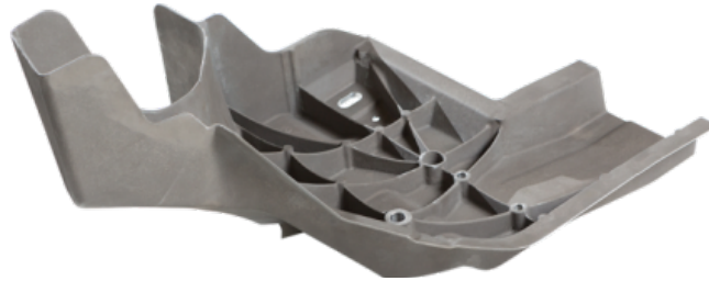
Figure 95 507lbs AE42 shipped to Vehma. Figure 96: MMLV Front Kick Down Rail.
