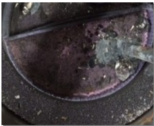
Figure 43. 180g of metal adhered to cathode
