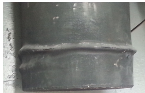
Figure 24. Beta 1.1 Damaged Casing
