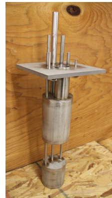
Figure 672: Gen II corrosion electrolysis setup
