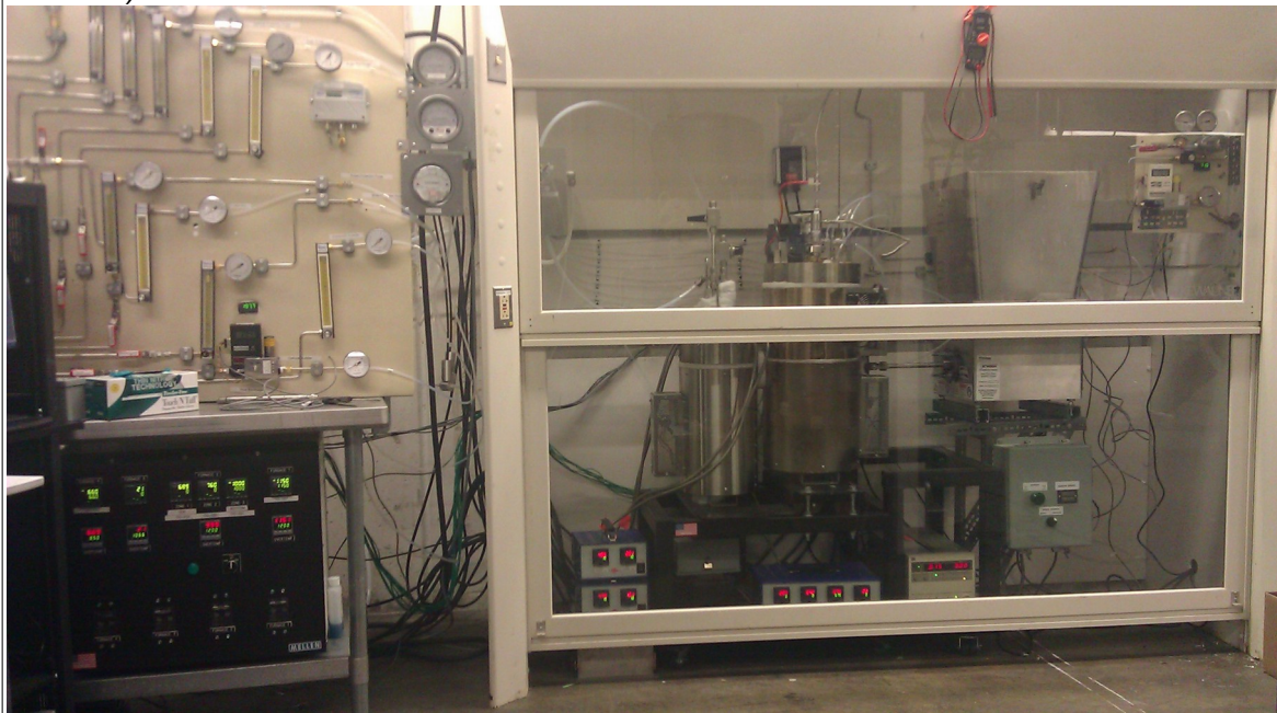
Figure 10: INFINIUM alpha magnesium production prototype in fume hood (right) with gas panel (upper left) and furnace power supply (lower left). New this quarter are the raw material augur and hopper system (to right of crucible), anode gas treatment system (upper right in fume hood), and new gravity cast mold (below crucible).
