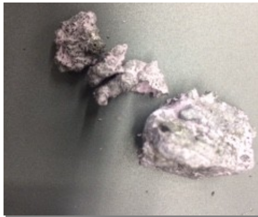
Figure 44. 50g of metal harvested by cooling the bath to solidify the metal and keep the salt molten
