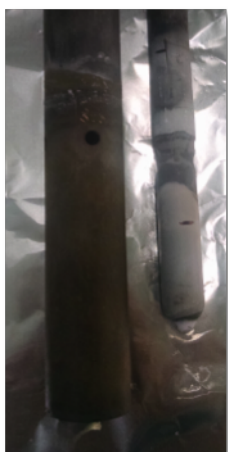
Figure 89 Offset purge cathode cage & YSZ membrane
