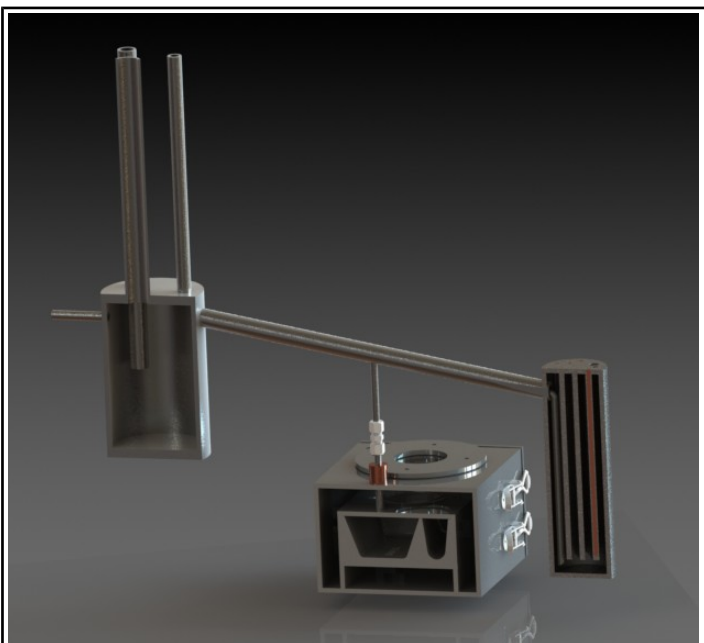
Figure 7: Rendered cross-section of crucible (left), condenser (right), and pour box (center) of alpha system.
