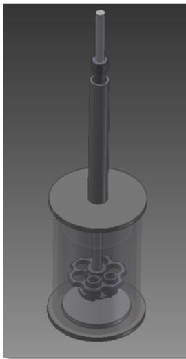
Figure 76 "Revolver" six-sample static test device.
