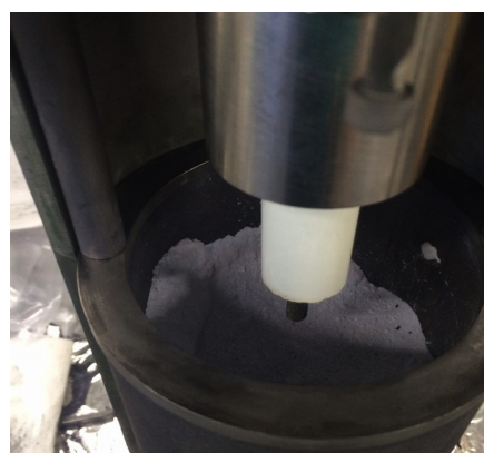
Figure 40. Open ended cathode sheath.
