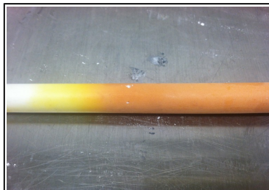
Figure 58: Candidate low-cost anode material diffusion through zirconia.
