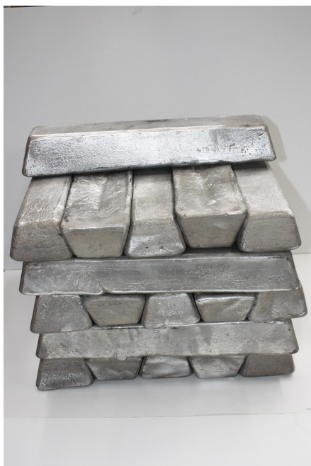
Figure 56 270lbs of AE42 produced using INFINIUM hardener
