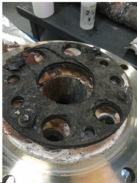
Figure 55: 304 baffles after 1 month of electrolysis
