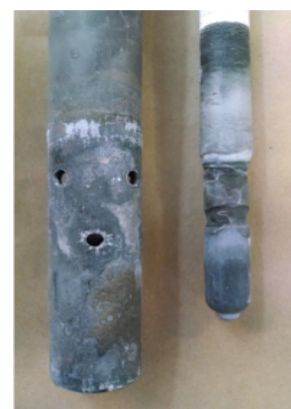
Figure 85 Cathode cage and zirconia tube post electrolysis
