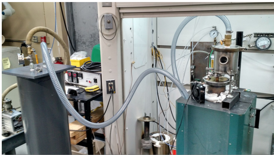
Figure 48. Molten Metal Siphon, aka the Lunar Landing Module
