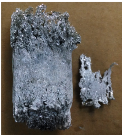
Figure 15 Mg recovered from Alpha 4.0 condenser
