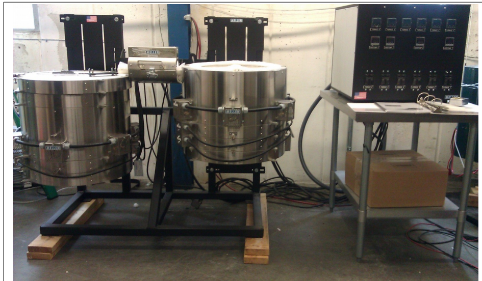
Figure 21: Modular furnace for INFINIUM beta magnesium production prototype cell, with two main 12" (30.5 cm) ID chambers for the crucible and condenser. and power supply on
