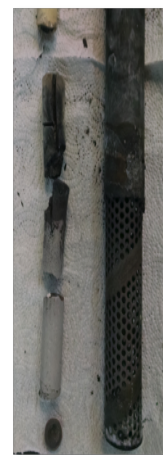
Figure 88. Zirconia Tube & Cathode Cage Post-Electrolysis
