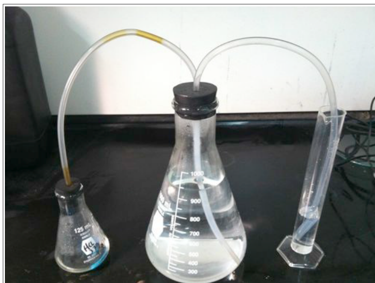
Figure 64: Apparatus for testing magnesium metal content of process salt.
