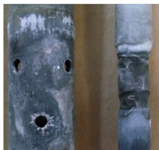
Figure 16 Cathode cage holes correspond to YSZ membrane degradation.
