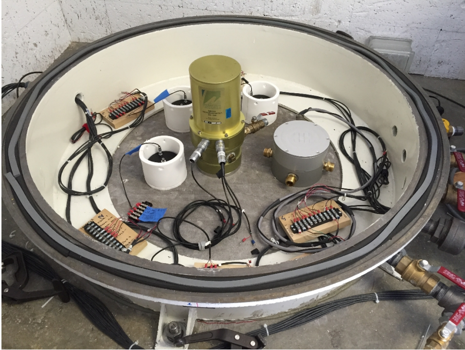
Figure 3 M-60 infrasound sensors encapsulated in white foam jackets, the MB2000 reference sensor, and a Hyperion 5113GP (not utilized during this evaluation)
