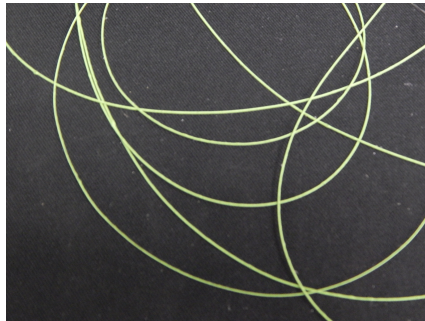
Figure 16: Green GI-POF Produced Using NanoSonic's Polymer Fiber Draw Tower System.
