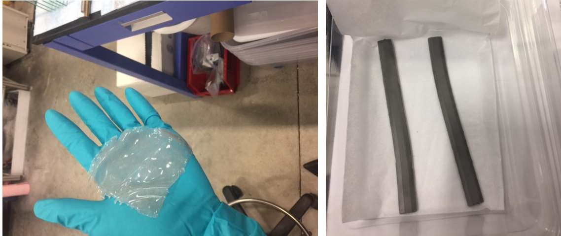
Figure 24: GaIn/Polymer Composite Systems. GaIn Liquid Metal was dispersed in NanoSonic's Custom Siloxane Polymer System at 14 (left) and 30 (right) Weight Percent.
