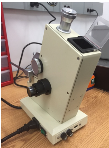
Figure 11: NanoSonic's Abbe Refractometer.
