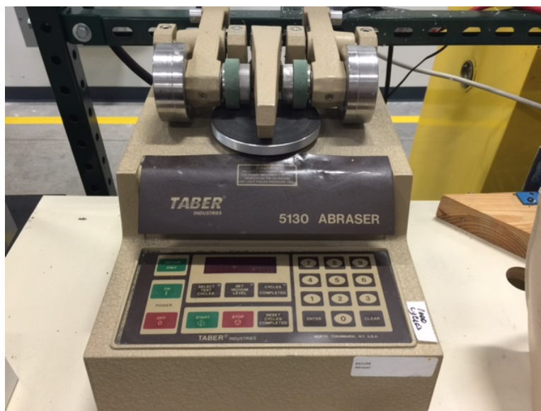
Figure 9: NanoSonic's Taber Abraser.
