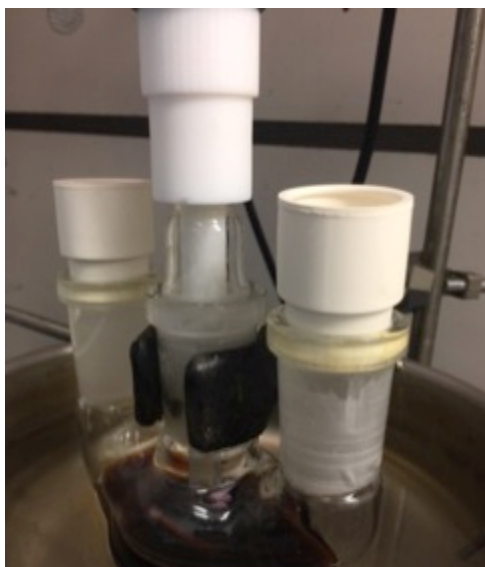
Figure 31: Custom Synthesis of Ultra-High Temperature, UV-Curable Polyimide Resin System.
