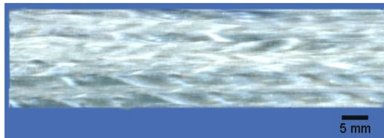
Figure 13. Aligned strand structure
