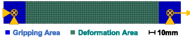
Figure 3: Macroscale bar model. The BCs are applied to each node in the gripping area
