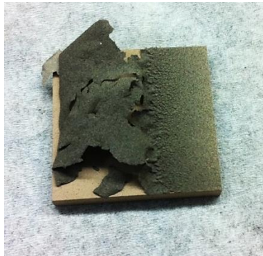
Figure 4.13. Photograph of oxidized thermal spraying ( \text{ZrSi}_2 coating) at 700 °C air for 10 hours. Coating delamination was clearly identified.
