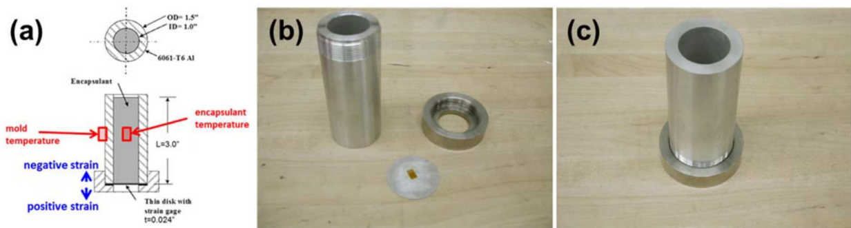
Figure 2-2. Thin-Disk-on-Cylinder (a) schematic, (b) individual parts and (c) assembled structure.
