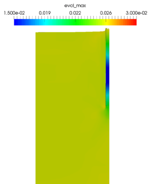
Figure 20: Maximum compressive volumetric strain shown in (a) front view (b) plan view and (c) sliced midway through the pile anchor R2L2.
