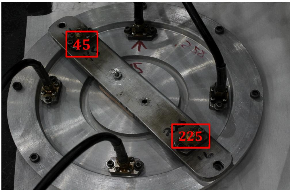
Figure 6. Back surface of the bin front plate. In this photo the four B-dots measuring the beam current (IBEAM) are connected with the diagnostic cables, the Ion B-dots are not connected. The numbers indicate the ion B-dot location. The beam four B-dots are located at the front surface of the plate and measure the current emitted from the cathode tip while the two ion B-dots should measure the back-streaming ion current striking the aluminum bar.
