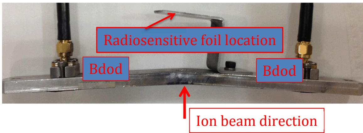
Fig. 8. Ion B-dot holder with both covered with aluminum foil
