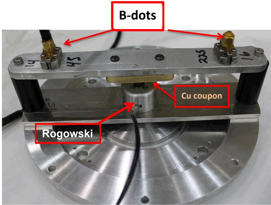
Figure 3. Bdot ,Rogowski coil and copper coupon arrangement mounted at the back of the knob front flat plate (first measuring station).
