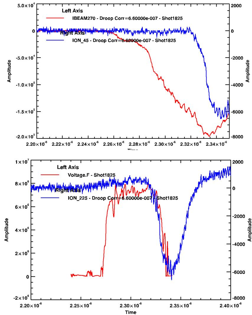
Fig. 16. The beam (IBEAM) current peak (200kA), the ion B-dot trace maximum and the A-K voltage collapse happens at the same time at approximately 2.34  $\mu$ s. The start of the voltage trace estimated at location F is corrected for the travel time of the retrapping wave from the diode to the F location.
