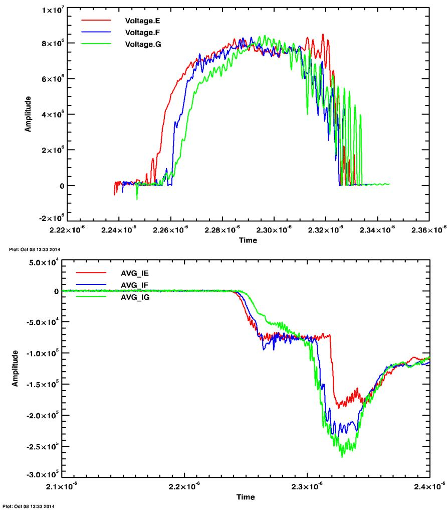
Fig. 17. The bound currents at location F (IF), G (IG) and E (IE) showing the retrapping wave propagating upstream follow the diode voltage collapse. The different voltage traces are calculated utilizing the parapotential formulas at
