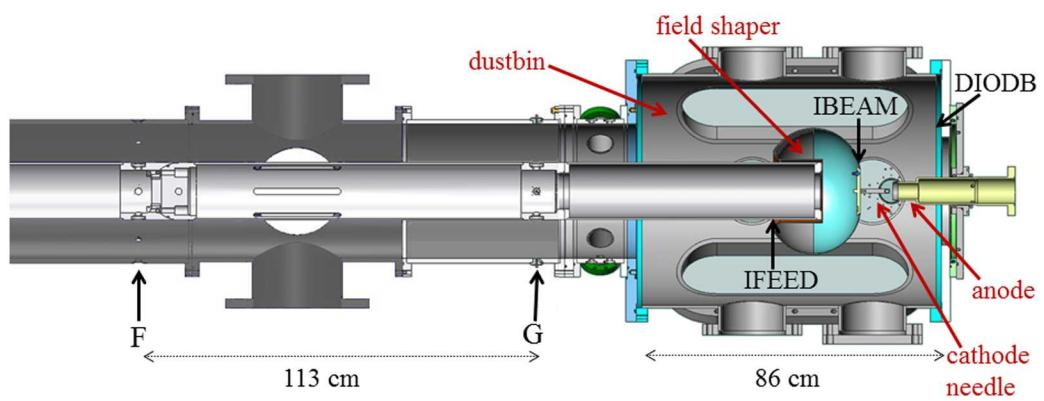
Fig. 17. Drawing of the Cathode stalk MITL indicating the location of B-dots measuring the current flowing along the cathode at different locations(F , G, IFEAD) upstream of the A-K gap.
