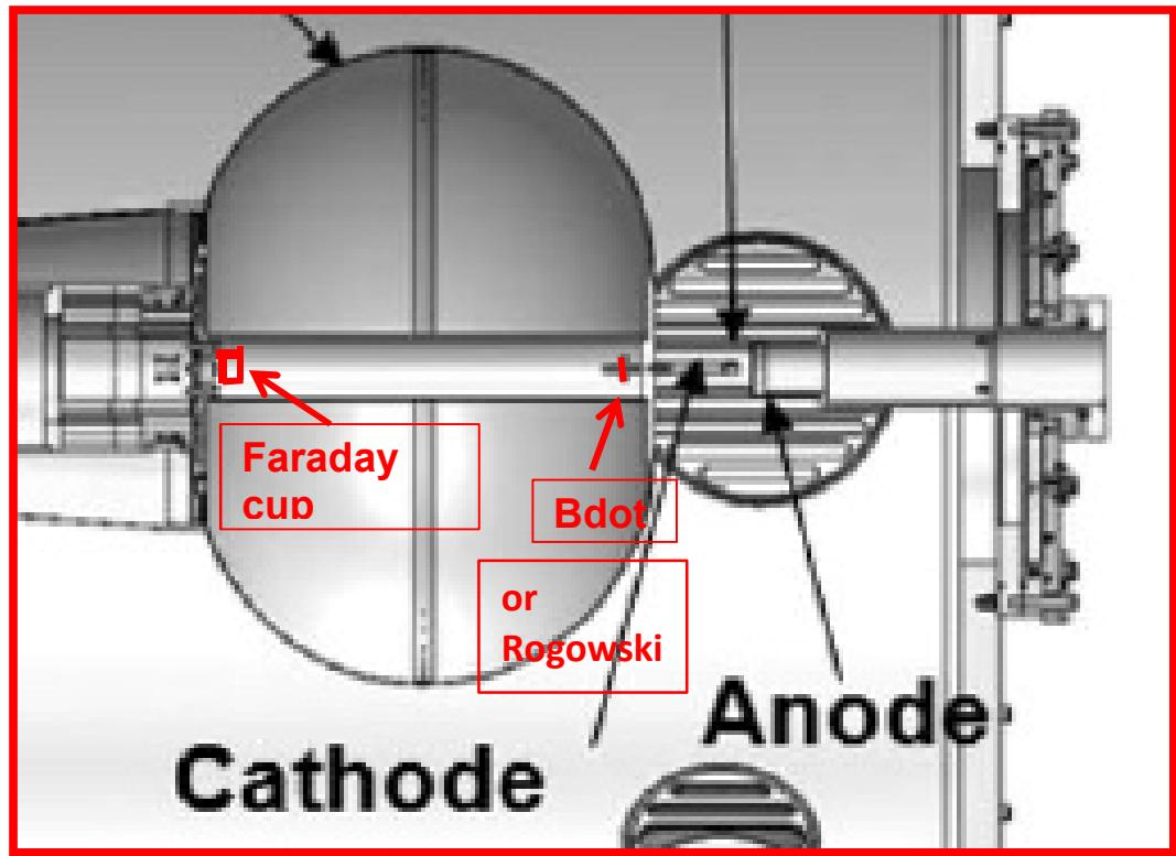
Figure 2. The engineering design of the dustbin indicating also the possible locations of Bdots and Faraday cup.
