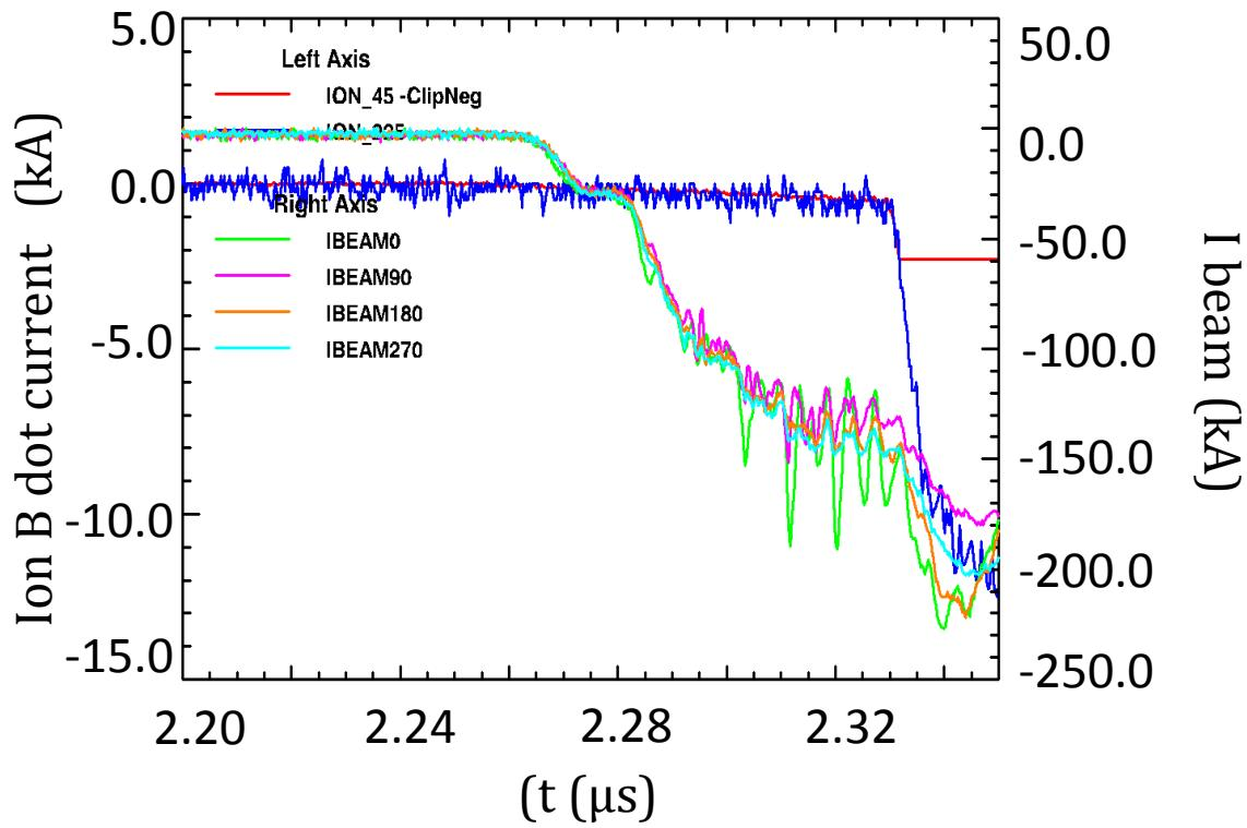
Figure 5. Shamble of the first results obtained with the B-dots at the first measuring station just on the back surface of the front plate. The ion B-dot #45 because of the large signal was clipped by the scope.
