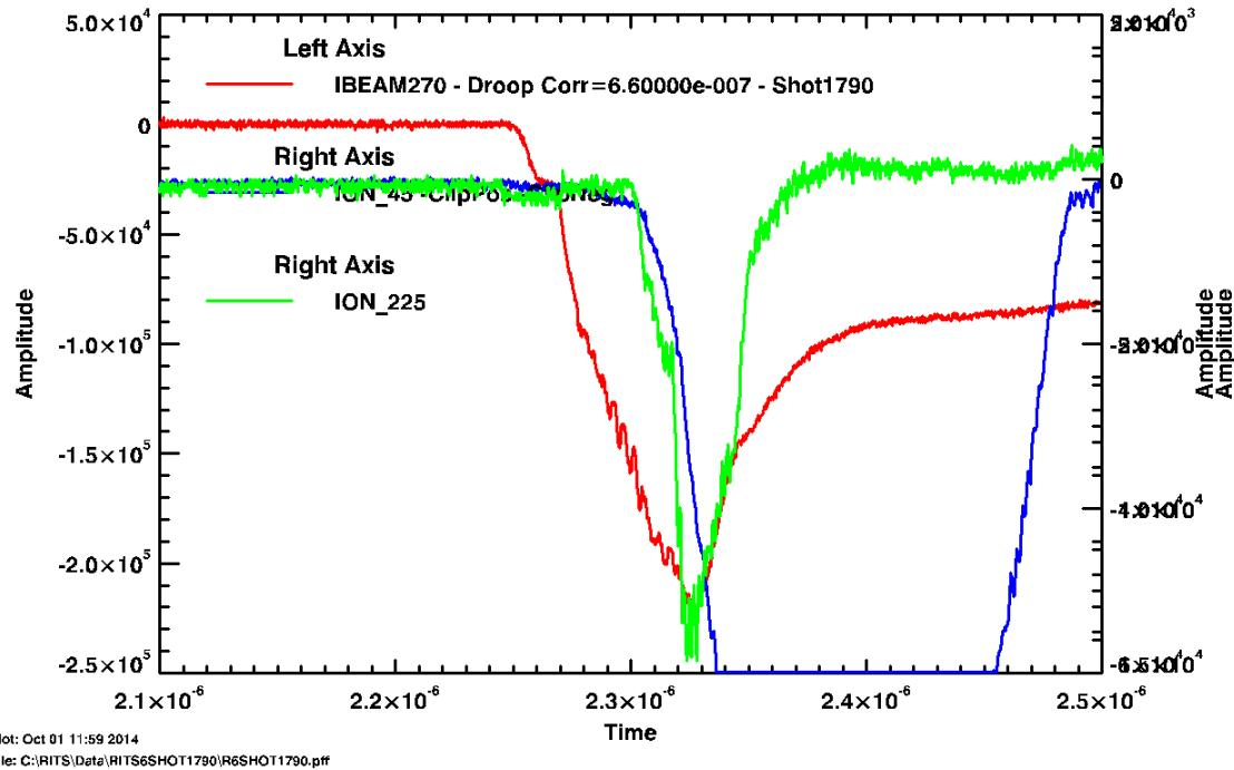
The signal is enormous and starts at the same time as when there was not the 50' cable. So the cable loop picks-up a lot of charge inside the knob. Also the pulse duration is much longer.
