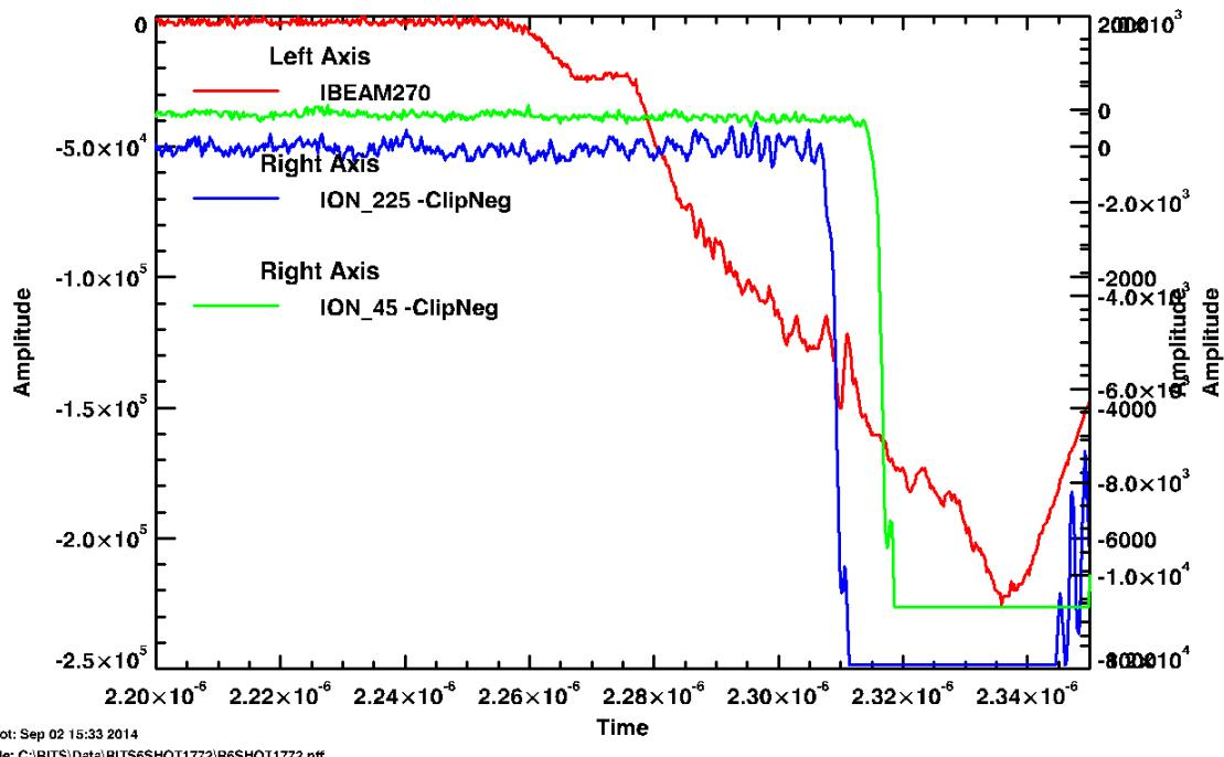
Fig. 11. One of the B-dots (#45) was rotated  $180^\circ$ . The “current” should have changed polarity. To no avail, as shown both B-dot signals appeared with the same polarity and same intensity
