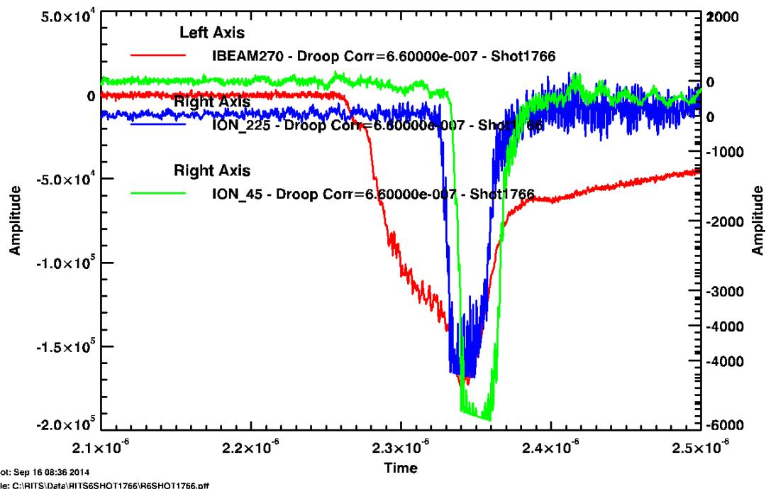
Fig. 9. Shot 1766. Both B-dots, the aluminum covered as well as the uncovered, showed the same polarity signal. Actually the covered B-dot (#45) registered even higher amplitude of "current".
