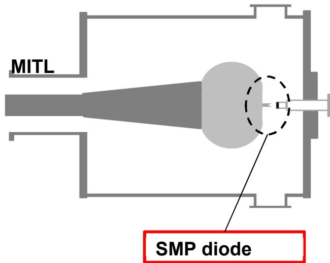
Figure 1. A schematic diagram of the RITS vacuum chamber (dustbin) and SMP diode. The relative dimensions are approximate.
