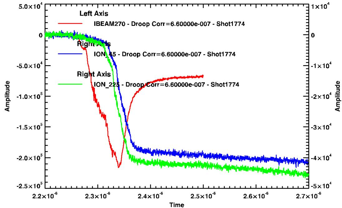
Fig. 13. Here we disconnected the cables from the B-dots and left them open (not shorted). The integrated signals appeared at the scope as step functions because the cables did not have a path to discharge to ground.
