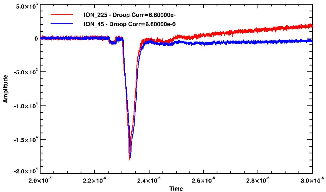
Fig. 15. In this shot we shielded the section of the cables located inside the knob with a 0.5 mm thick aluminum and stainless steel pipes. This did not reduce or eliminate the observed signals.
