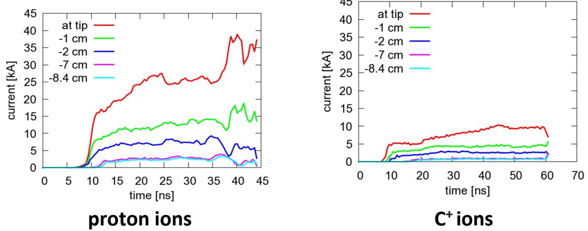
Fig. 7. LSP simulations of the back-streaming proton and carbon ions. In these simulations the cathode stalk length (needle), 8.4 cm, and the inner diameter, 1 cm.
