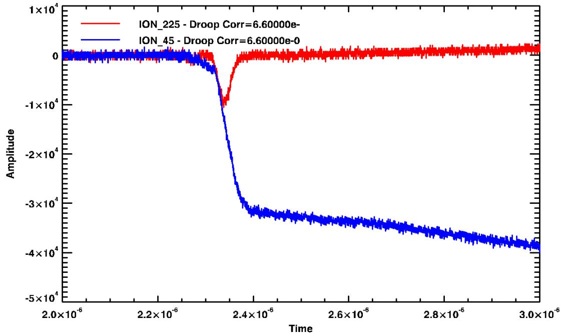
Fig. 12. We disconnected the diagnostic cables from the B-dots and shorted the end of one of them (# 225). The signal of #225 cable appeared similar to a B-dot while cable #45 gave a strong negative step function. Both signals started at the same time in synchronism with the diode collapse.
