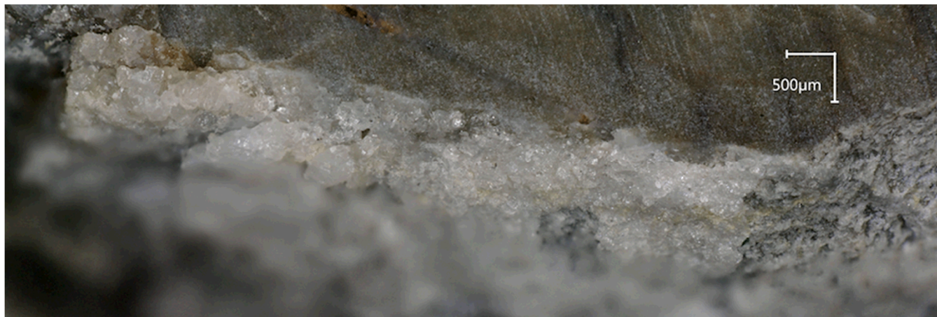
Figure 6. Magnified view of colorless surface particles shown in Figure 5. The granular nature and size of the colorless particles are visible in this image. XRF measurements were made near the center area of this photo. Please see Figure 7.
