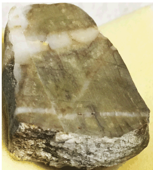
Figure 5. Quartzite rock sample, after cutting with rock saw. XRF measurements were performed perpendicular to the cut surface over an area that included the cut edge of the laser-processed face [facing down in this photograph] and exposed bulk quartzite from the cutting.
