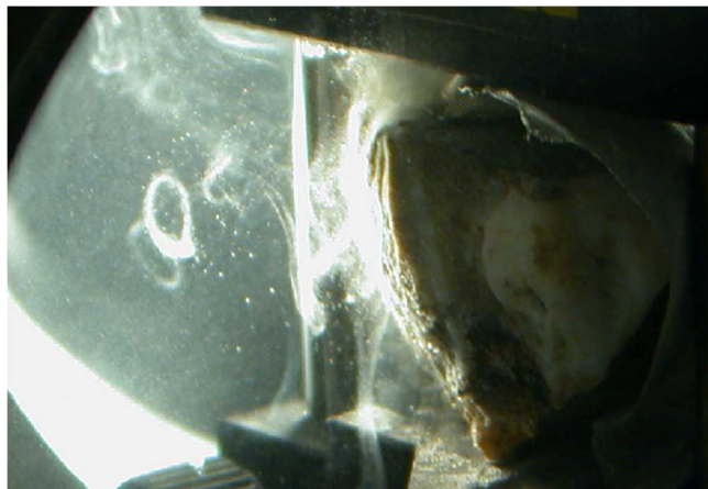
Figure 2. Photograph of side-view of quartzite sample, submerged in deionized water, shortly after laser pulse struck surface, releasing a cloud of sub- \mu\text{m} particles. Laser beam entered from the left, cloud was released towards the left.
