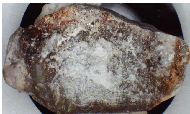
Figure 3. Photograph of dried quartzite sample, after 100 pulses of 527-nm, 1.8-J/pulse at \sim 0.6 \text{ J/cm}^2 , showing dramatic loss of color in laser-treated surface.
