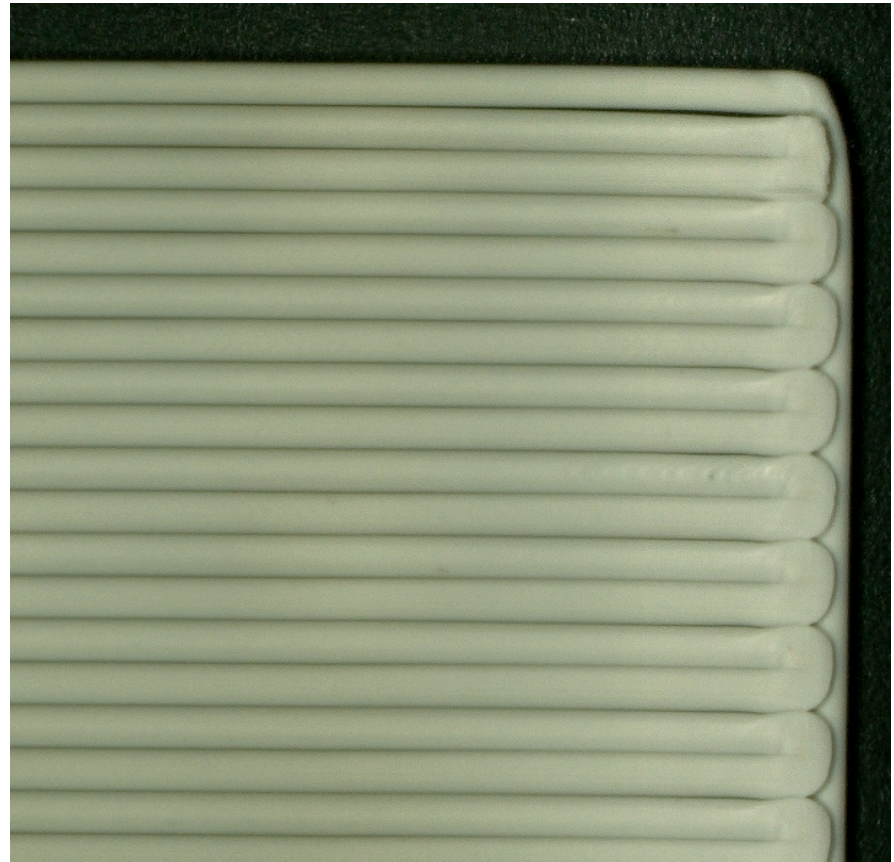
Direct write printed polymer-alumina specimens in the green state.
