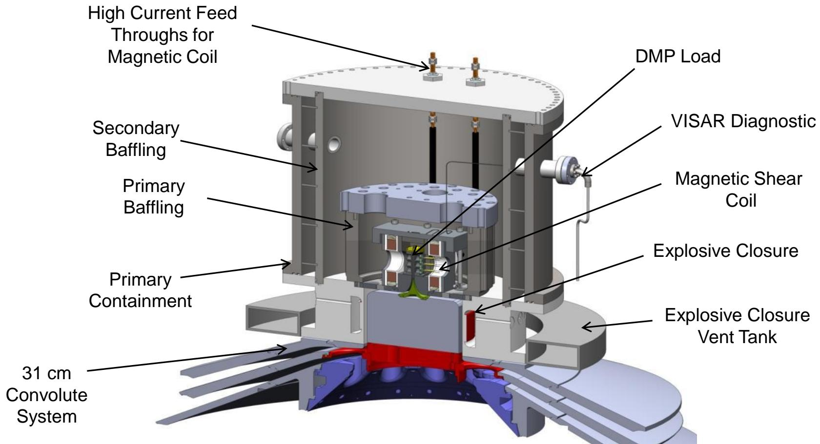
**DMP Load with Magnetic Shear**
