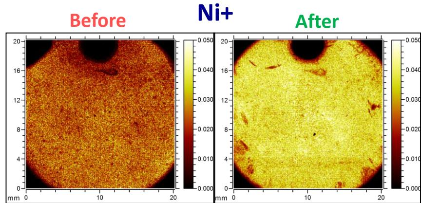
Coupon with environmental exposure survey, shown **Before** and **After** plasma cleaning. Increase in detected bulk nickel indicates reduced surface contaminants on SS304 sample.
