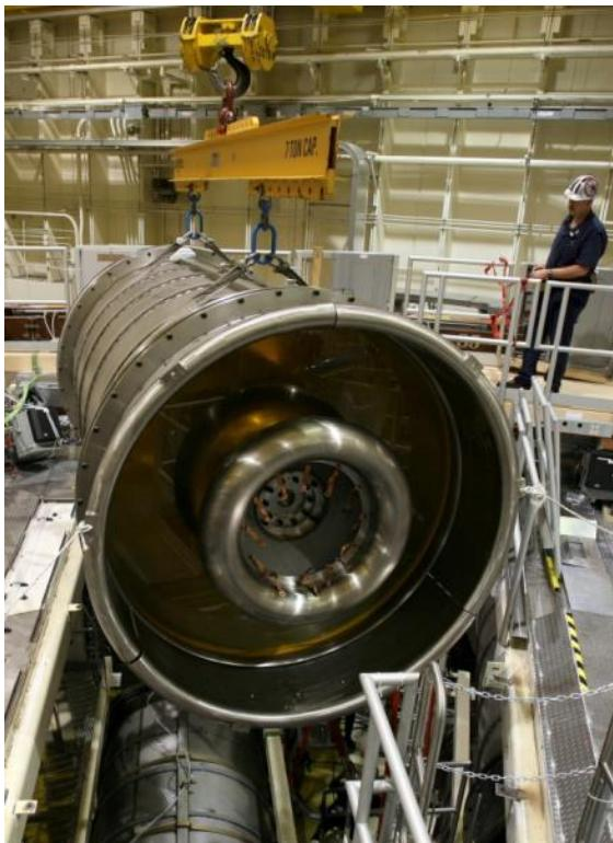
Inspection of a Marx Trigger Generator (MTG)
