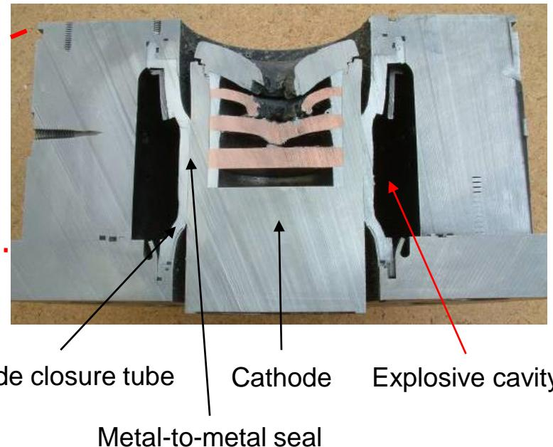
We have a proven containment system for Pu experiments used many times
