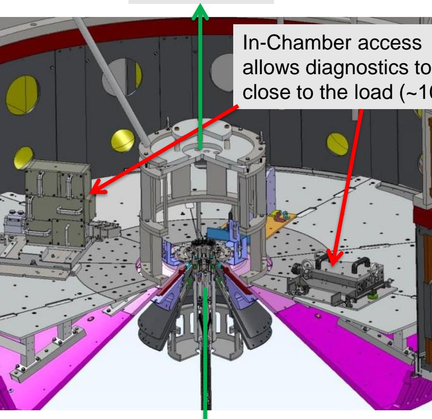
18 Radial Line-of-Sight Access Ports at  $12^\circ$
