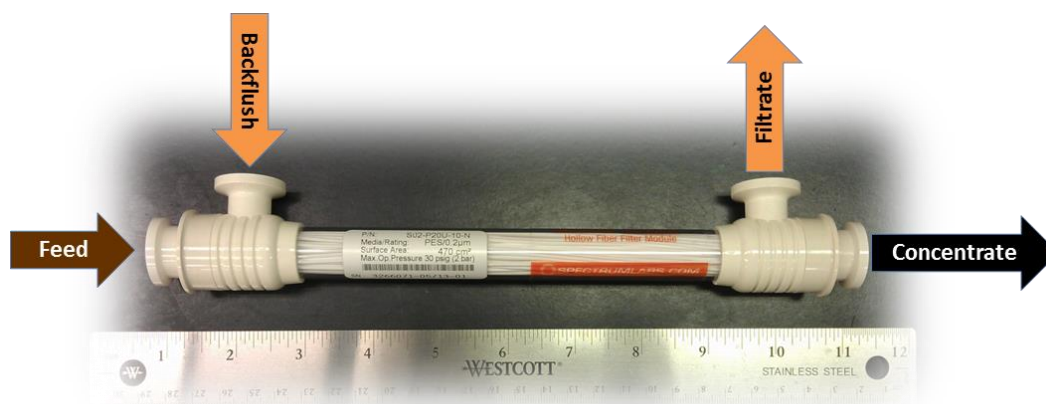
Figure 8.1.18 Commercial hollow fiber membrane module
