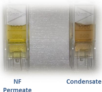
Figure 8.2.14 Photograph of NF permeate and condensate (from pulp and paper mill evaporator)
