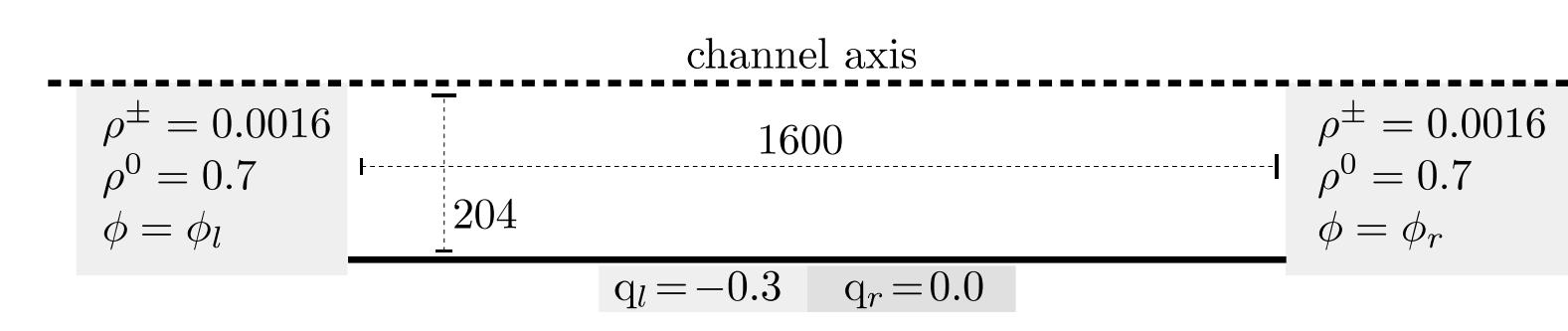
The channel occupies the middle of the domain, with a reflective boundary at the channel's axis for computational convenience. This allows us to model only half of the device. A comparison between the PNP, cDFT, and Hybrid anion density profile near the charged wall is given below for this application problem
