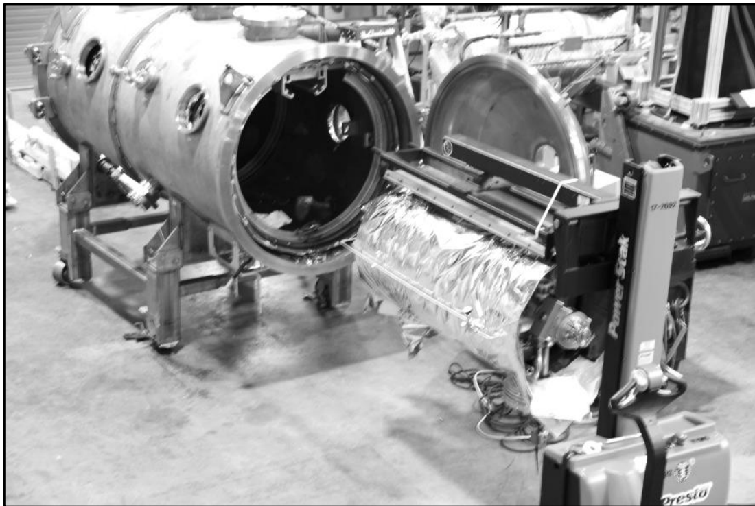
Figure 1. Cavity insertion into HTA using power lift.
