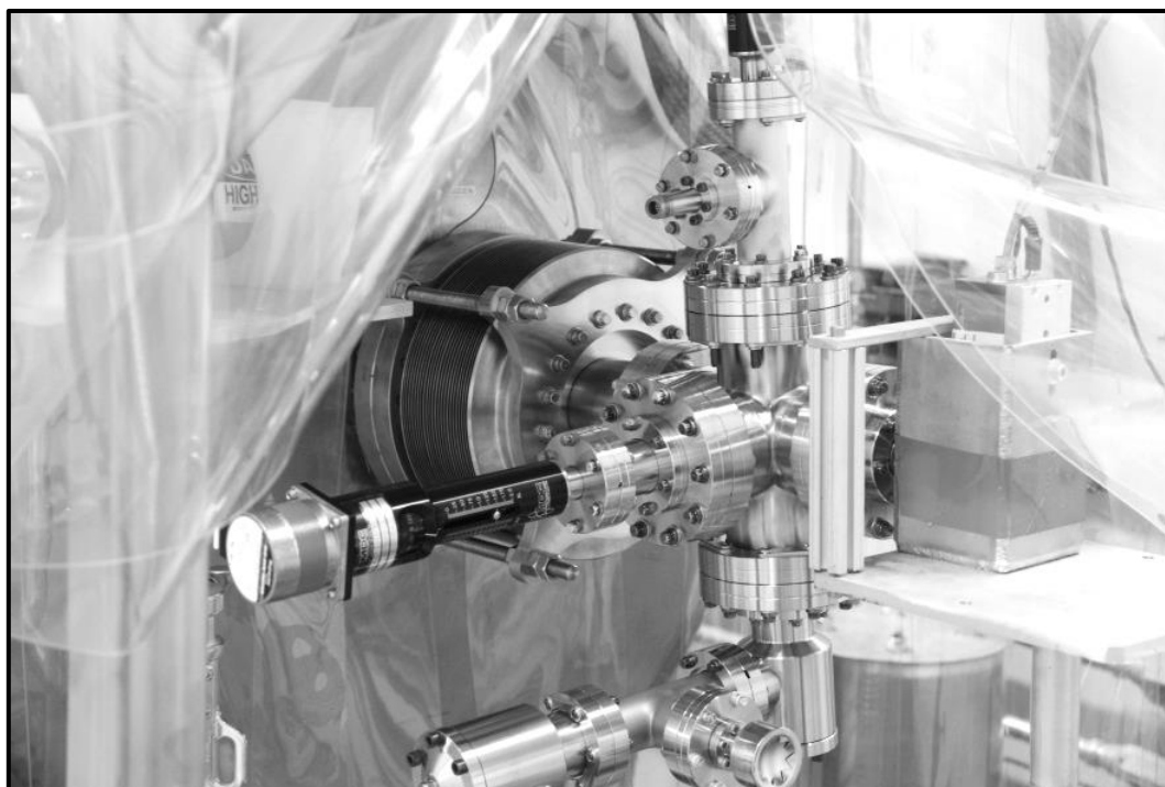
Figure 6. HTA beam tube cross and out warm to cold transition piece
