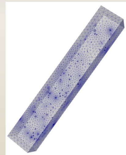
discretization & mesh of defect structure in dogbone A, 16 gage section
