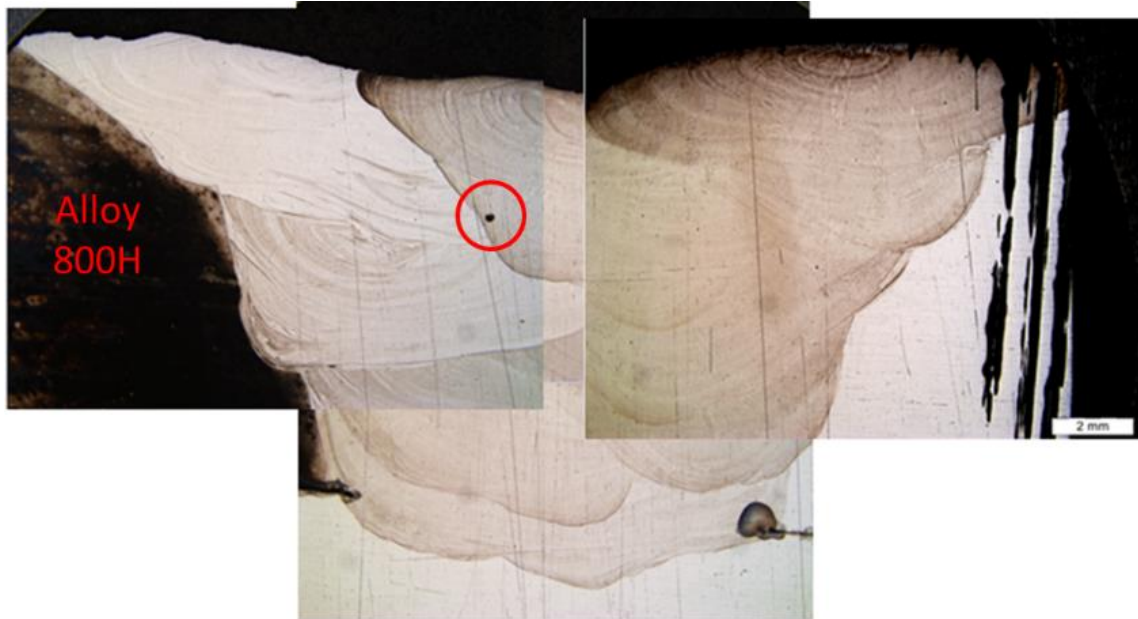
Figure 3. Macrograph of the second DMW showing no observable lack of fusion defects and one small gas pore (red circle)
